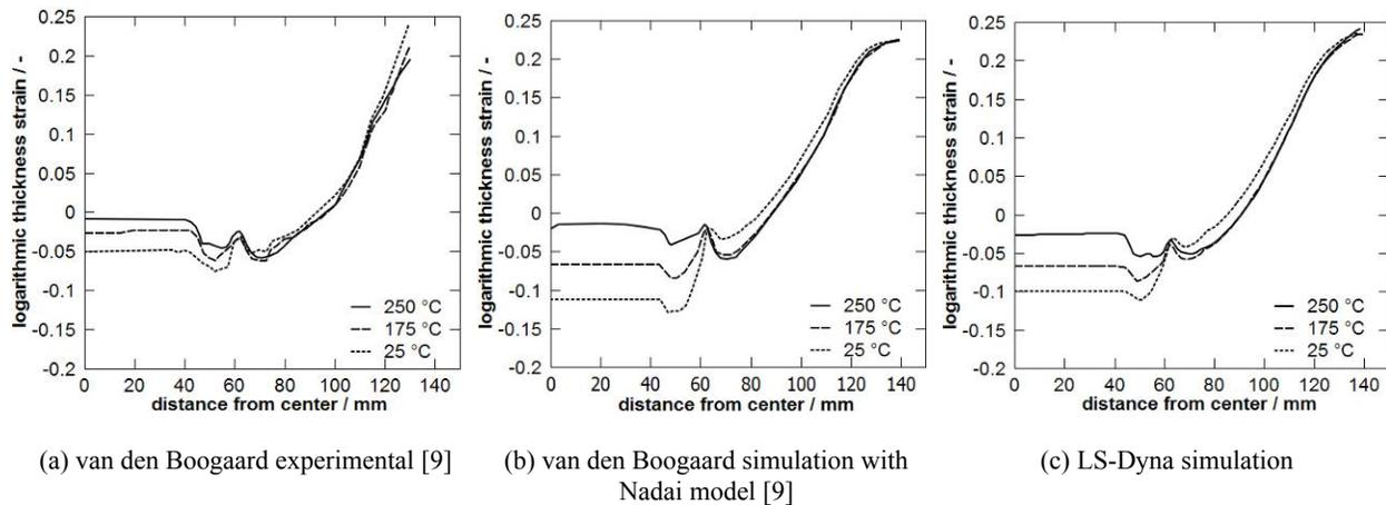
FIGURE 4. Experimental and numerical determined thickness distributions
