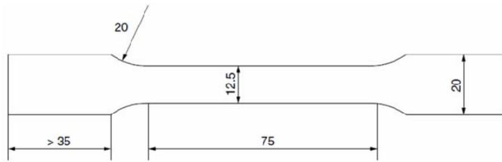
FIGURE 1. Geometry of the simulated tensile test specimen (dimensions in mm) [9]
