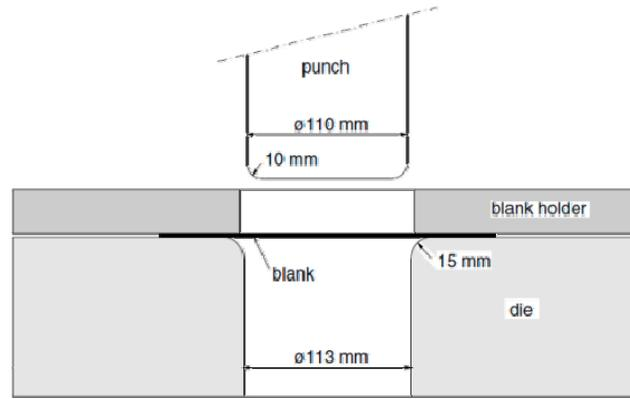
FIGURE 3. Geometry of the cup deep drawing example from literature [9]
