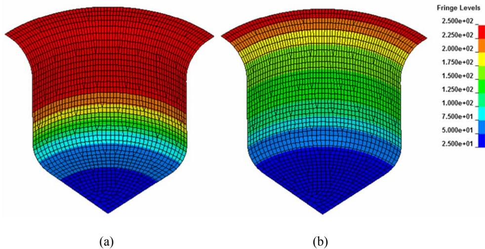
**FIGURE 6.** Numerically determined temperature distributions in °C after deep drawing at 250 °C flange temperature and 20 mm/s punch velocity (a) without and (b) with a cooled drawing radius
