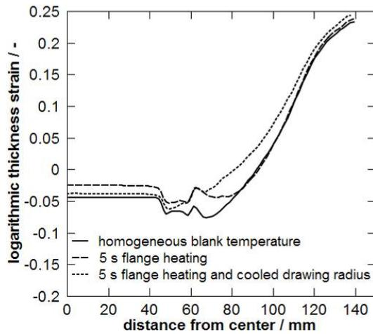
**FIGURE 5.** Thickness distribution results for different process layouts at 250 °C flange temperature and 20 mm/s punch velocity
