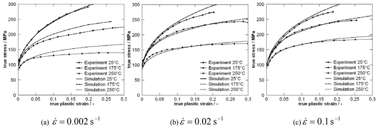
FIGURE 2. Experimental and LS-Dyna simulation results of the uniaxial tension test
