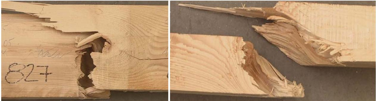
*Fig. 5: Low tensile strength due to local grain deviation caused by a broken tree-top (Spec.Nr.827)*
