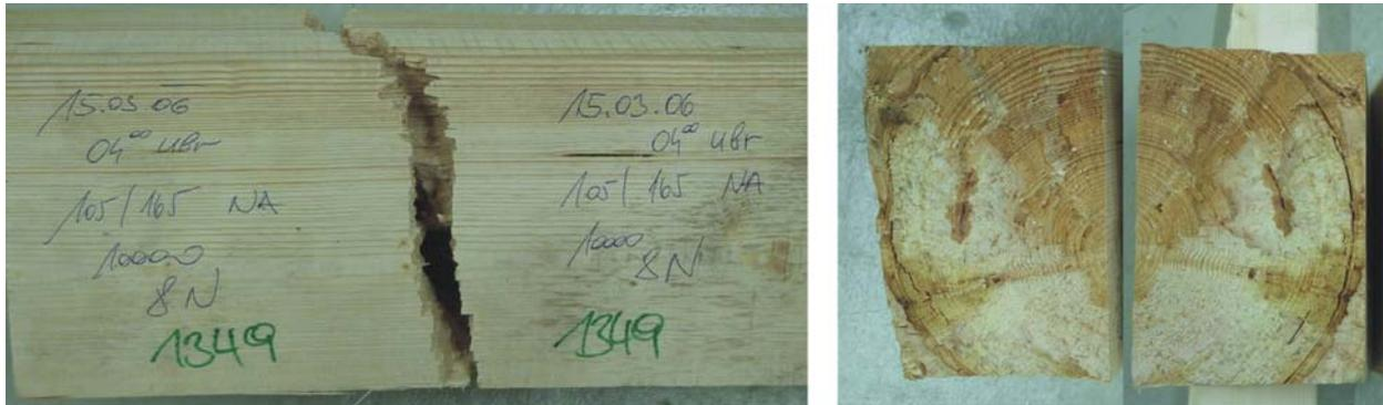
Fig. 7: Tensile strength = 6,37 N/mm<sup>2</sup> due to compression damage of the timber (Spec.Nr.1349)
