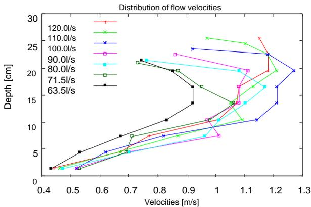
Figure 5: Velocity profiles in the chute at different discharges
