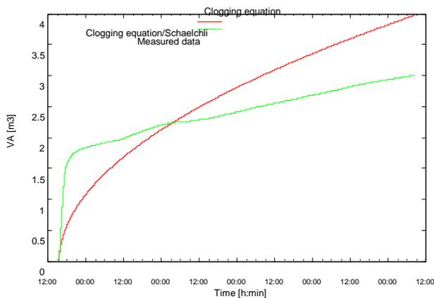
Figure 9: Volume of percolated water measured (test 3) and calculated
