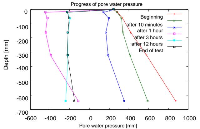
Figure 7: Gradient of pore water pressures at box 1 for test 3
