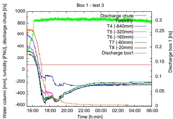
Figure 6: Turbidity, percolation water and pressures at box 1 for test 3
