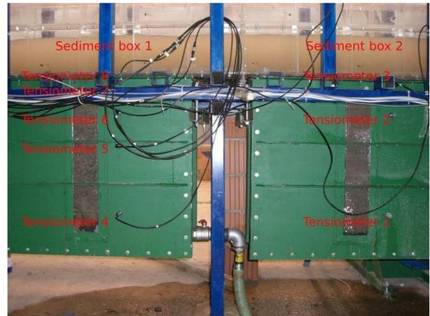
Figure 4: Arrangement of the tensiometers within the sediment boxes
