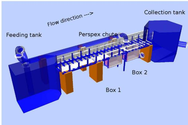
Figure 2: Test facility, 3D view
