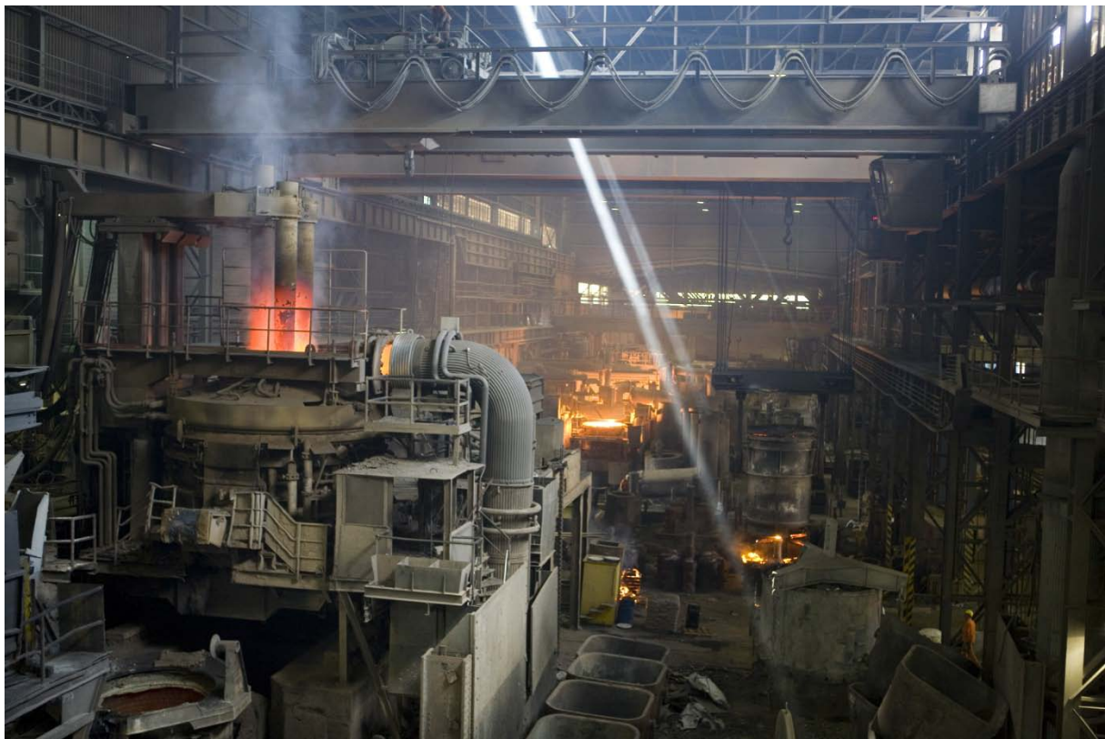
Fig. 1 Breitenfeld melt shop with EAF in the foreground
