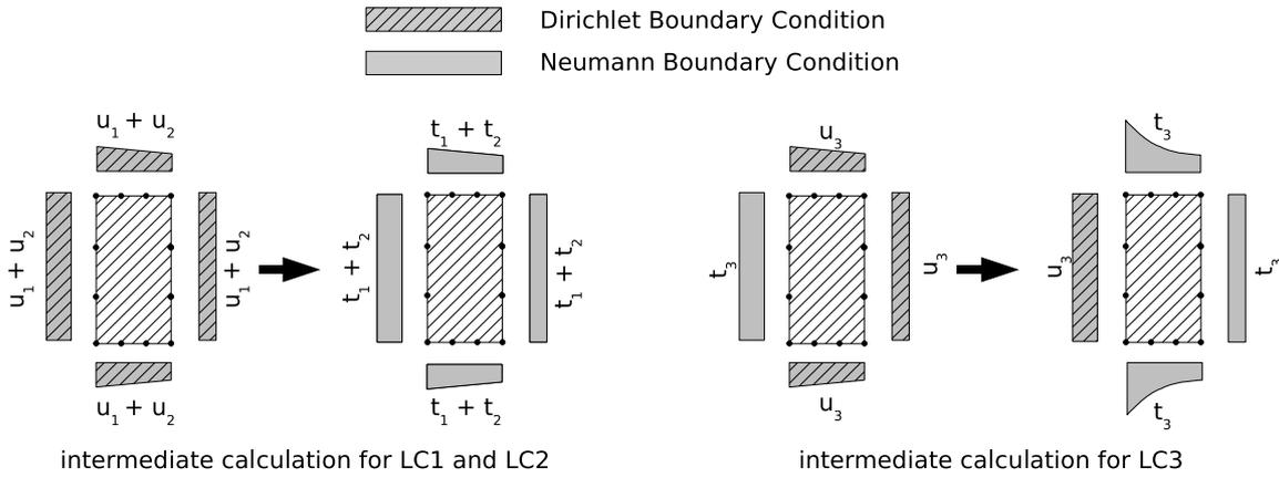
Figure 7: Intermediate calculation for LC1, LC2 and LC3
