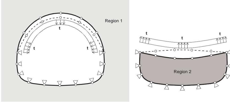
Figure 2: Fixed interface nodes and given boundary conditions at free nodes
