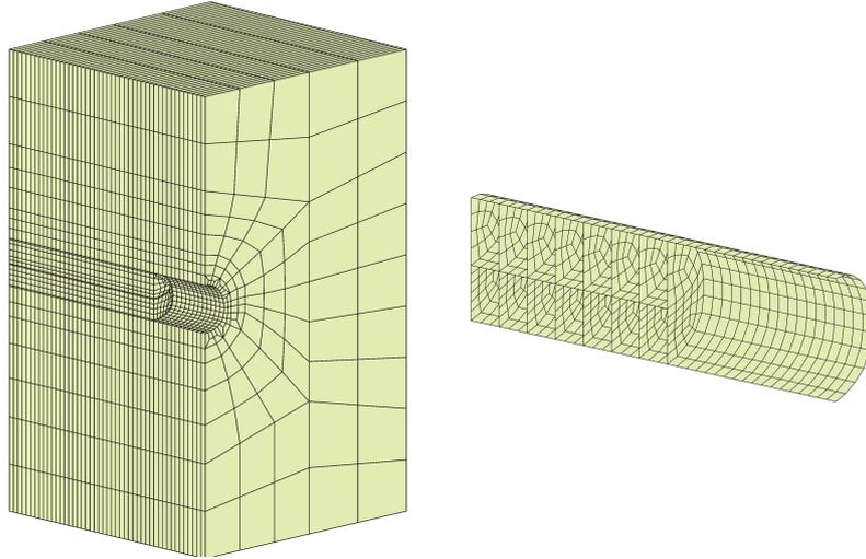
Figure 3: Finite element mesh (left) - boundary element mesh (right)
