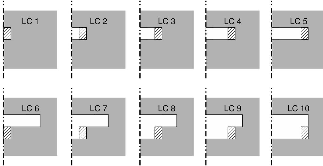
Figure 5: Longitudinal tunnel section - sequence of all load cases
