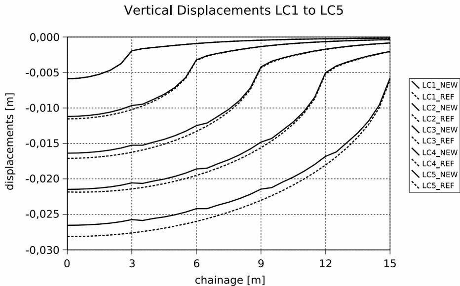
Figure 10: Vertical displacements at tunnel crown
