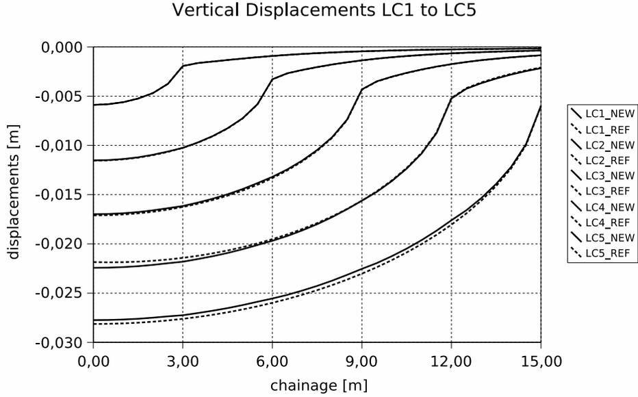
Figure 8: Vertical displacements at tunnel crown
