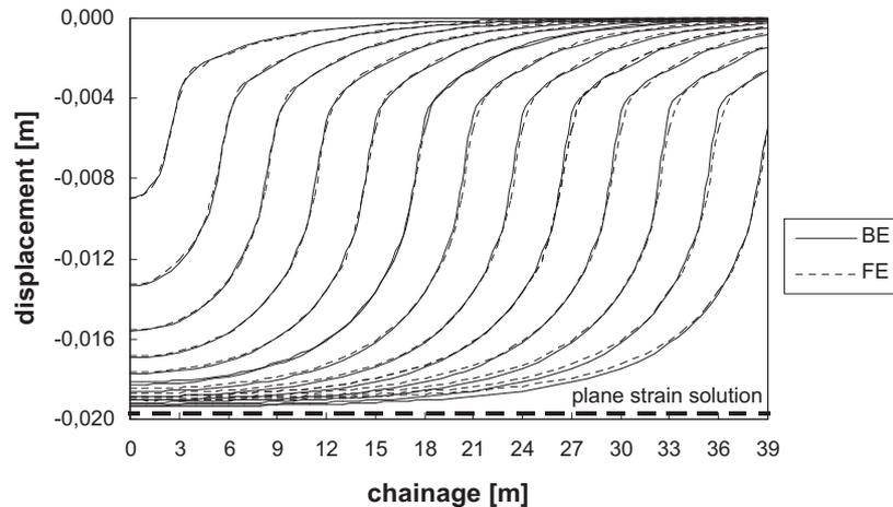
Figure 4: z-displacements at the crown of the tunnel for 13 load cases
