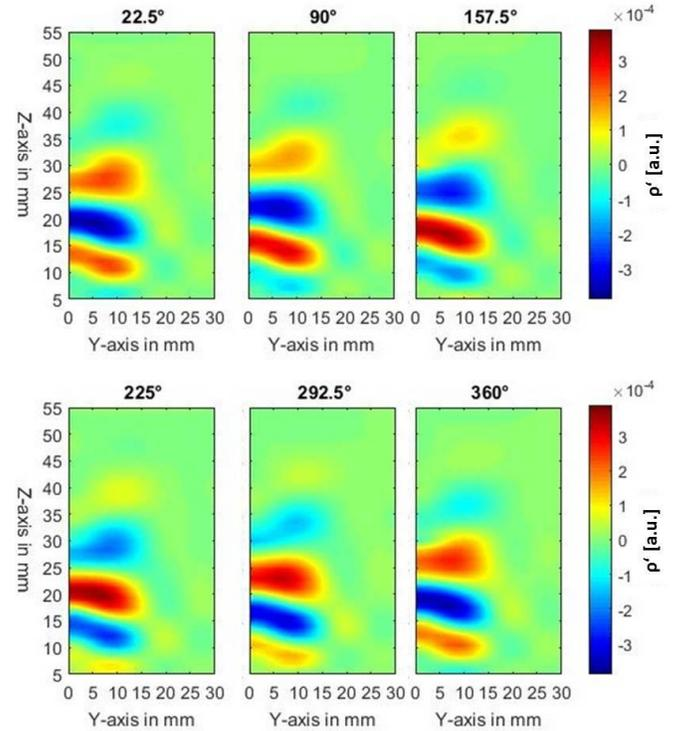
FIGURE 6: PHASE RESOLVED LOCAL DENSITY FLUCTUATIONS AT 212HZ ALONG THE JET AXIS Z, PLOTTED IN RADIAL DIRECTION Y
