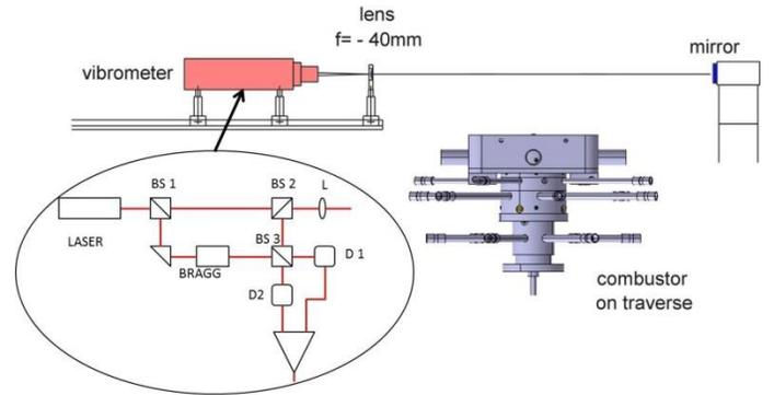
FIGURE 2: EXPERIMENTAL SETUP FOR LIV MEASUREMENT: VIBROMETER, LENS, BURNER, MIRROR; BOTTOM LEFT: PRINCIPLE FUNCTION OF A LASER VIBROMETER: BS... BEAMSPLITTER, L... LENS, D... DETECTOR
