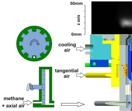
FIGURE 1: EXPERIMENTAL SETUP OF THE BURNER FOR PERFECTLY PREMIXED OPERATION OF THE SWIRL-STABILIZED FLAME; AXIAL AIR AND FUEL ARE ALREADY MIXED BEFORE ENTERING THE BURNER; AXIAL AIRFLOW IS MODULATED WITH A ROTATING DISC (SIREN) SHORTLY BEFORE ENTERING THE BURNER. THE FLAME IS INDICATED BY THE CORRESPONDING MEAN OH\* EMISSION.
