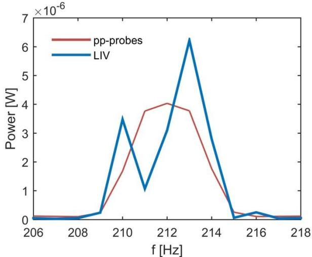
FIGURE 7: COMPARISON OF SOUND POWER OBTAINED FROM PP-PROBES COMPARED TO THE SOUND POWER FROM LIV MEASUREMENT
