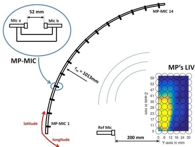
FIGURE 3: LEFT: MICROPHONE ARRAY, CONSISTING OF 14 PP-PROBES (TOP LEFT) WITH AN ANGLE OF 6 DEGREE BETWEEN EACH PROBE. RIGHT: 2D-MEASUREMENT GRID OF THE LIV: LINE OF SIGHT INTEGRATED DENSITY FLUCTUATIONS REPRESENTING THE AVERAGE SHAPE OF THE FLAME; THE POSITION OF THE REFERENCE MICROPHONE IS SHOWN IN THE MIDDLE
