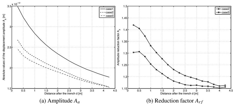
Figure 4: Displacement amplitude  $A_a$  and the corresponding amplitude reduction factor  $A_{rf}$
