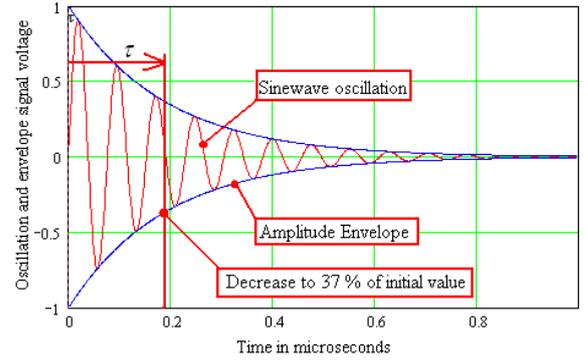
Figure 11. Attenuated harmonic sine wave oscillation as impulse response of a parallel resonant circuit of Q-factor 8.
