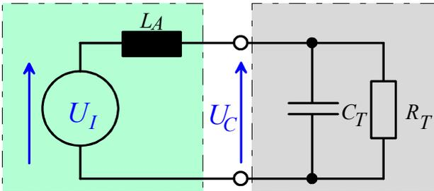
Figure 2. Transponder equivalent circuit for power considerations.
