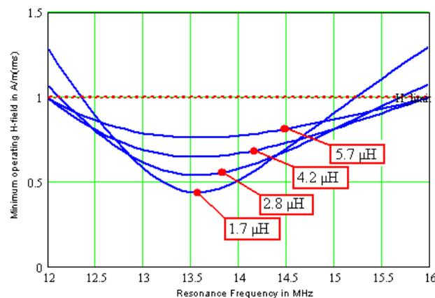
Figure 8. Minimum  $H$ -field for start of chip operation as function of resonance frequency, antenna inductance  $L_A$  as parameter.
