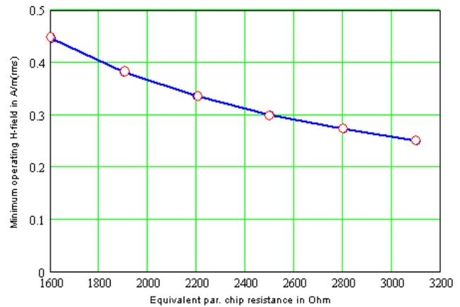
Figure 7. Minimum  $H$ -field for start of chip operation as function of equivalent parallel transponder resistance  $R_T$ , for resonance at carrier frequency.
