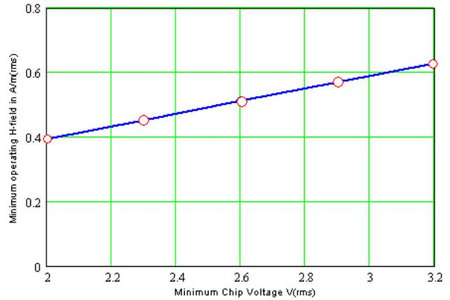
Figure 5. (Required) minimum  $H$ -field for start of chip operation as function of minimum chip voltage, for resonance at carrier frequency.
