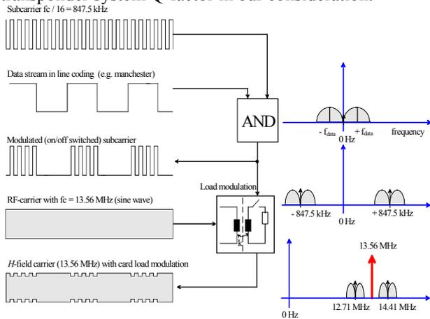
Figure 12. Loadmodulation principle according to [13], modified.
