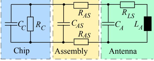
Figure 3. Transponder equivalent circuit for chip, assembly, antenna.
