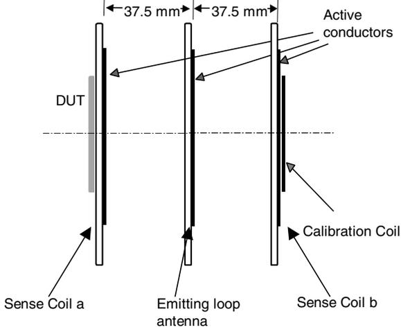
Figure 1. Coax. antenna assembly for contactless transponder test [2].
