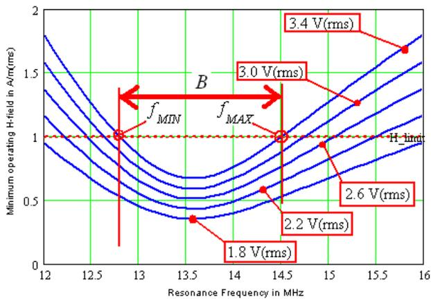
Figure 4. (Required) minimum  $H$ -field for start of chip operation over resonance frequency, minimum chip voltage  $U_{CMIN}$  as parameter.
