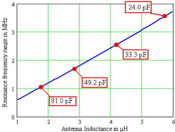
Figure 10. Relation between antenna inductance and allowable resonance frequency tolerance range.
