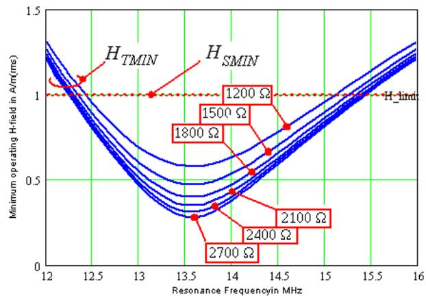
Figure 6. Minimum  $H$ -field for start of chip operation as function of resonance frequency, equivalent parallel transponder resistance  $R_T$  as parameter.
