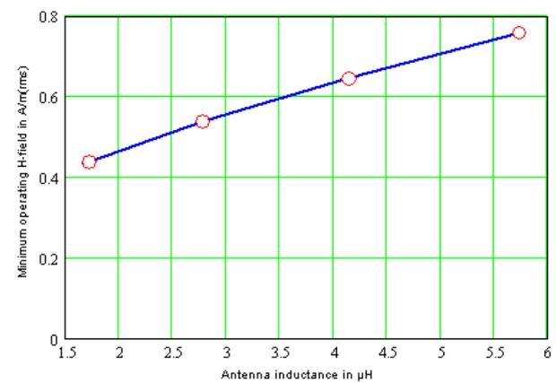
Figure 9. Minimum  $H$ -field for start of chip operation as function of antenna inductance  $L_A$ , for resonance at carrier frequency.
