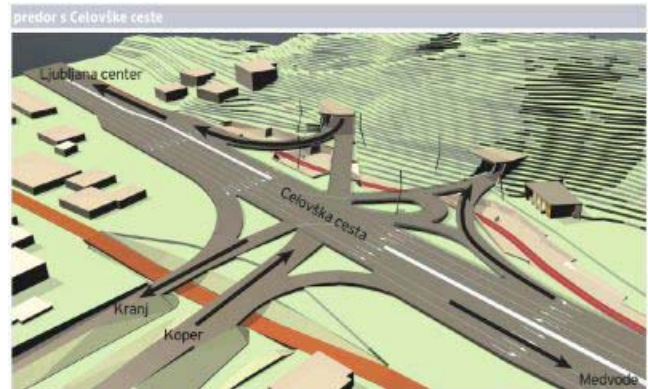
North portal of Šentvid tunnel: first 400m are old and new galleries; the rest is tunnel trough a hill.
