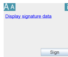
Fig. 5. The GUI provided by MOCCA Online's Java Applet allows users to review data to be signed and to start the signature creation process.
