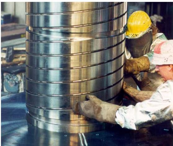
**Figure 1:** Shrink-fitting of a liner holder
