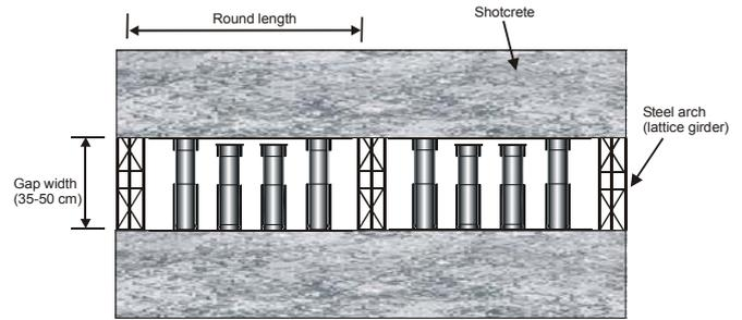
Fig 11. Typical assembly of LSC groups between steel arches
