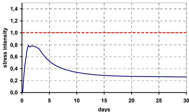
Fig. 14. Development of the stress intensity factor for the same rock mass conditions, but with higher advance rate
