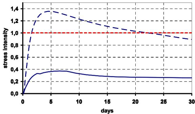
Fig. 13. Development of stress intensity factor in the shotcrete lining without (dashed line) and with yielding elements (solid line)
