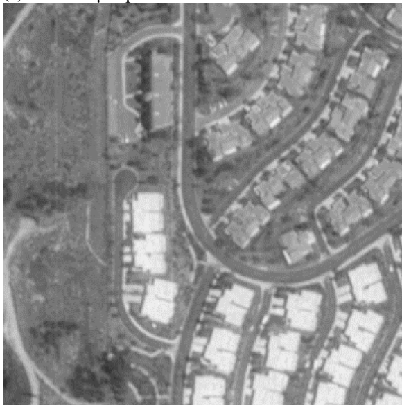
Figure 10: Segments of an aerial photograph used to create the DEMs in Figure 9. Scan resolution is 20 µm per pixel, but in (a), the pixels are obtained from the native resolution of 868 dpi, in (b) from 5000 dpi. Area is about 180 m x 180 m .
