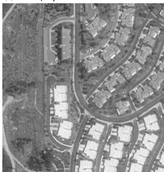
Figure 10: Segments of an aerial photograph used to create the DEMs in Figure 9. Scan resolution is 20 µm per pixel, but in (a), the pixels are obtained from the native resolution of 868 dpi, in (b) from 5000 dpi. Area is about 180 m x 180 m .
