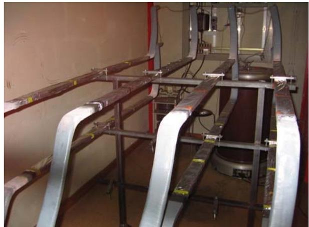
Figure 6: Test Set-Up for Generator bars
