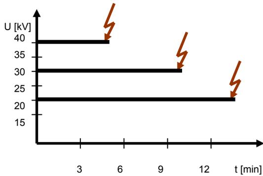
Figure 4: long-time breakdown tests with characteristic loads
