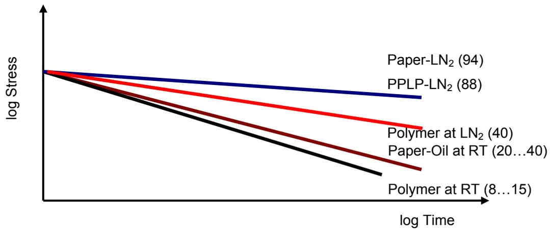
Figure 7: Lifetime curve of different insulation systems, measured and literature of cryogenic and room temperature (RT) insulation systems
