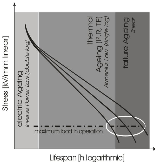
Figure 1: Aging processes, Lifetime in dependence of stress
