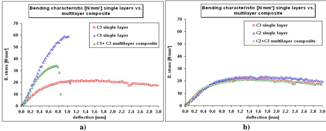
**Figure 14.** Bending characteristic of commercial single coating layers and their multilayer composites depending on a) rigid/soft and b) soft/soft
