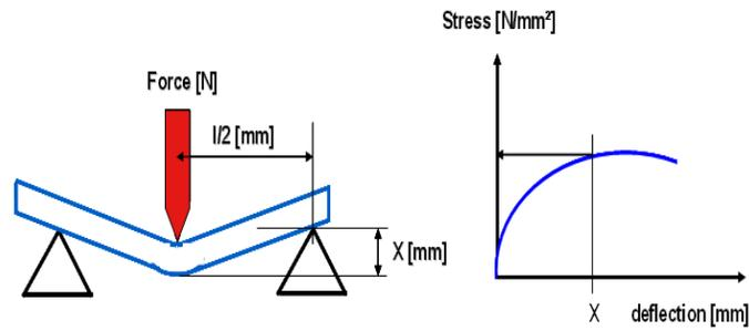
**Figure 3.** 3 point bending methodology and stress characteristic
