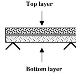
**Figure 2.** Layer definition of multilayer composite at bending measurements
