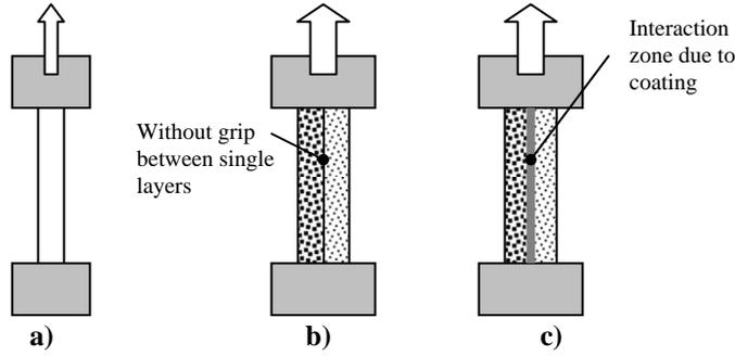
**Figure 1.** Types of in-plane tensile test samples
