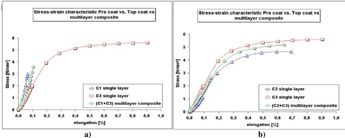
Figure 11. In-plane stress-strain characteristics of single layers and multilayer coating films based on commercial coatings a) C1 and C3 and b) C2 and C3
