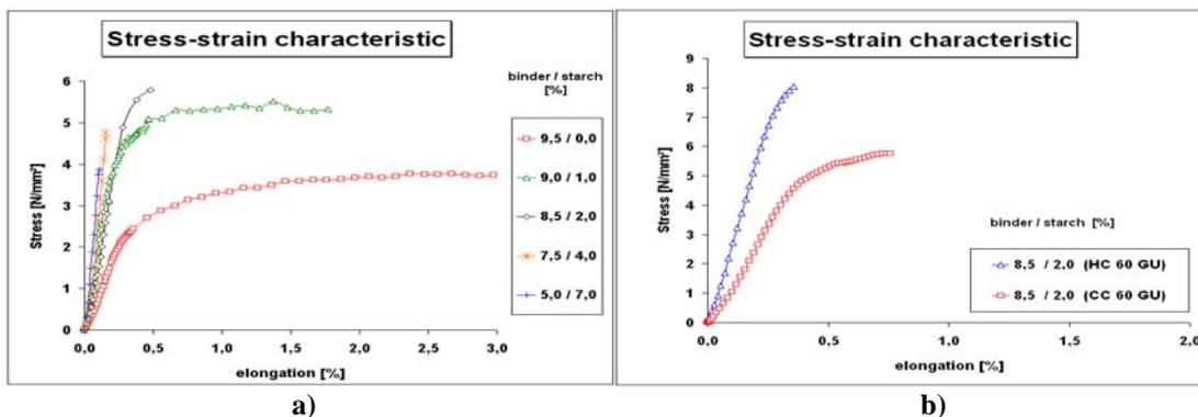
**Figure 5.** Stress-strain characteristic caused by a) latex exchange and b) pigment type exchange of single coating layers basing on latex-starch ratio (Dextrin A) and pigment particle size (Dextrin B)
