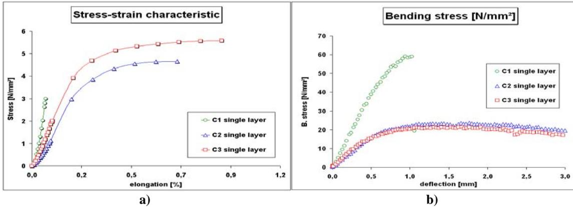
**Figure 8.** a) Stress-strain characteristic and b) Bending stress of commercial single coating layers
