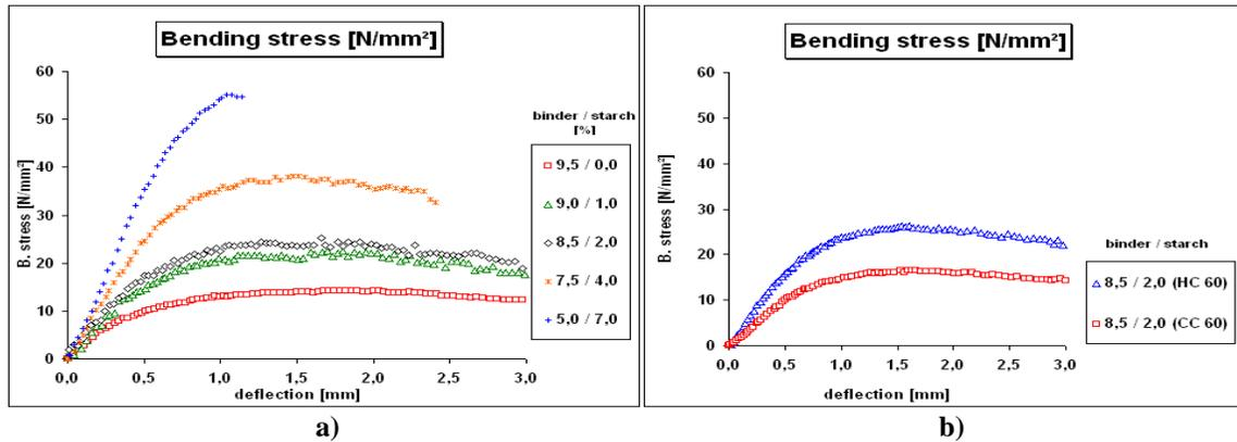
**Figure 6.** Stress-strain characteristic of single lab coating layers depending on a) latex-starch ratios and b) pigment type
