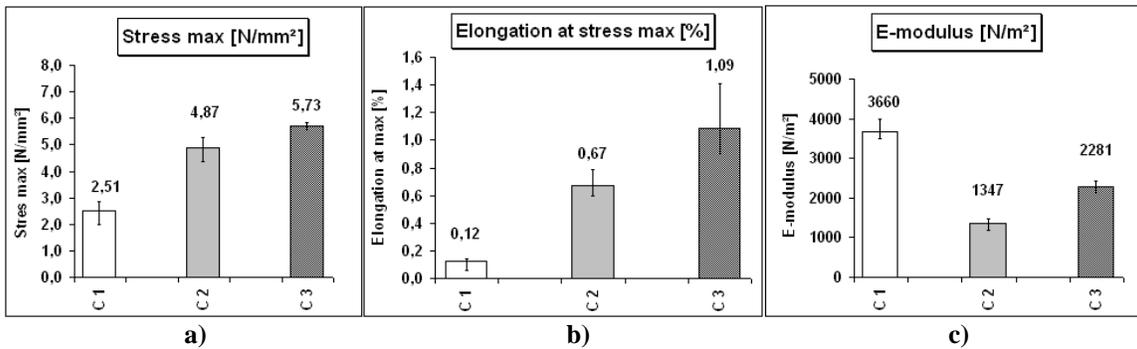
**Figure 7.** a) Stress maximum b) elongation at stress maximum and c) E-modulus of single coating layers of commercial coatings
