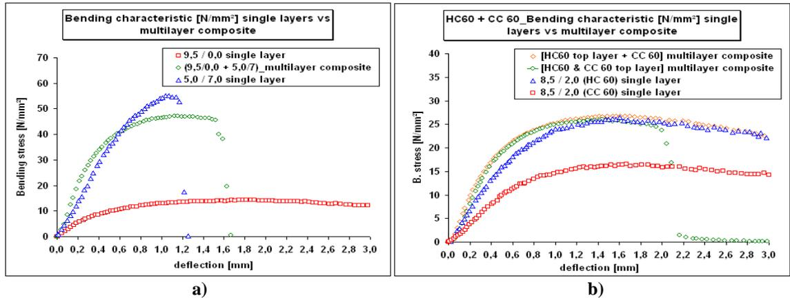
**Figure 13.** Bending characteristic of single coating layers and their multilayer composites depending on a) very rigid versus very soft behavior and b) pigment types
