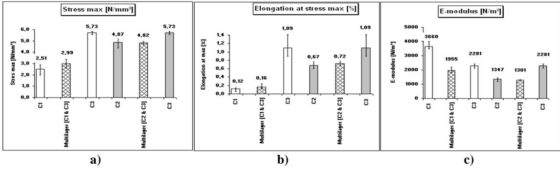
**Figure 12.** a) Stress maximum b) elongation at stress maximum and c) E-modulus of single coating layers and their multilayer composite of commercial coatings
