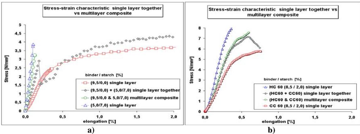
**Figure 9.** In-plane stress-strain characteristics of single layer, single layer together and multilayer coating films based on a) latex-starch ratios and b) pigment type
