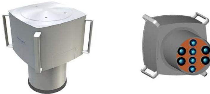
Figure 6: Overview of the UltraCam D large format digital aerial camera. A set of 8 optical cones exists holding a total of 13 CCD arrays to assemble a large format digital image in RGB-color and near infrared NIR. Multiple area array CCDs collect pixels. Each CCD array feeds signals into their own compact and proprietary electronics setup and data path. For dimensions and weight see Table 1.
