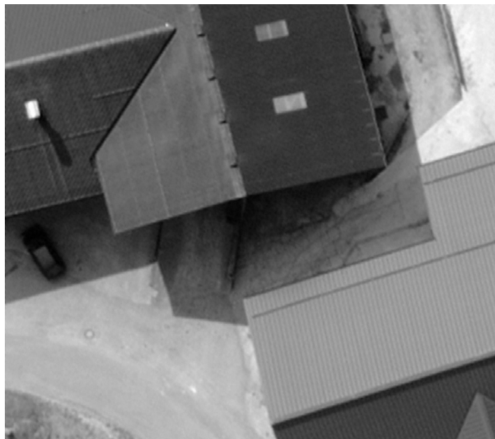
Figure 3: Detail from an UltraCam-image at a pixel size of 12 cm on the ground. Note the definition of the roof surfaces and the detail in the shadows.
