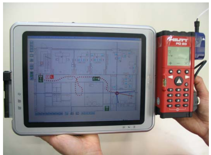
Figure 1. Prototype of a “gyro-laser-tracker“ based on an HP Tablet PC with a gyroscope and laser range meter
