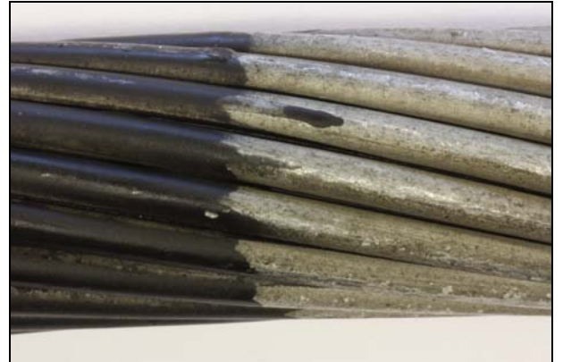
Figure 7: Macro of the used line (left coated, right bare)
