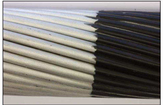
Figure 8: Macro of the unused line (left bare, right coated)
