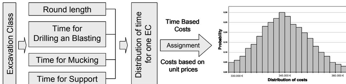
**Figure 4 Procedure to determine the distribution of cost and time for one Excavation Class**
