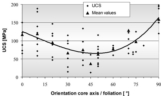
**Figure 2 Evaluation of laboratory test results**
