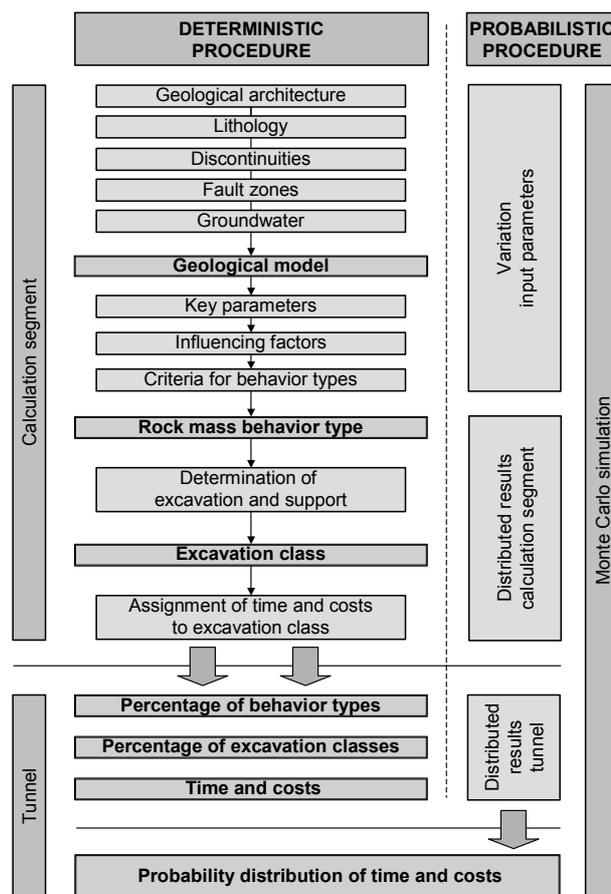
Figure 1 Procedure for the determination of the geotechnical risk
