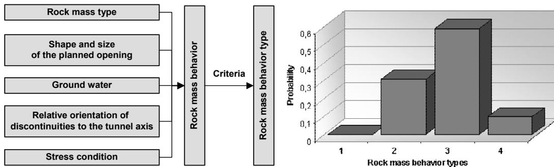
**Figure 3 Probability of occurrence of determined Behavior Types for one calculation segment**
