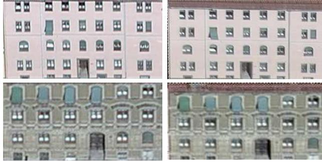
Figure 5: The marked sections of Figure 4 have been rectified. At left are two sections from the oblique data at 45°, at right from the vertical data at 27° .
