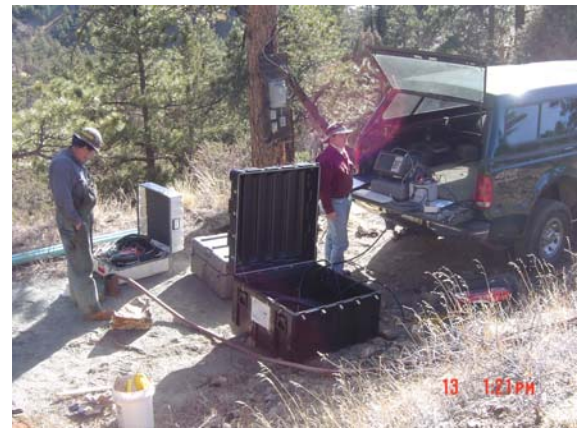
Fig. 13. Data acquisition setup, with water being added to borehole U1A.
