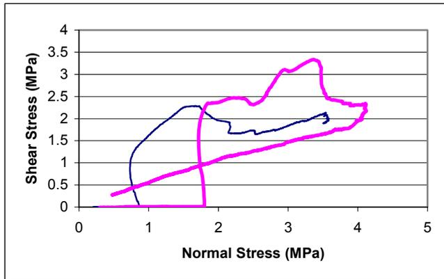
Figure 16. Mohr stress paths for the two tests performed under Infinite CNS parallel to the foliation, the thicker line represents the sample with a higher quartz content.
