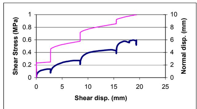
Figure 9. Stress displacement plot for the above test. Thick line is the shear stress while the thin line is the normal displacement. Note the drops in shear stress at higher stress levels related to the breakdown of the internal structure.
