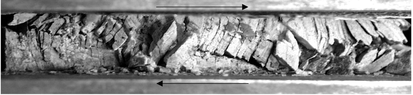
Figure 19. Sample after shearing 2 cm under infinite normal stiffness. Note the through going shear plane from upper left to lower right. Initial foliation was slightly against the shear direction which was dextral. The failure mode was bookshelf type shear. Sample size is approx. L = 13cm, H = 1.9 cm.
