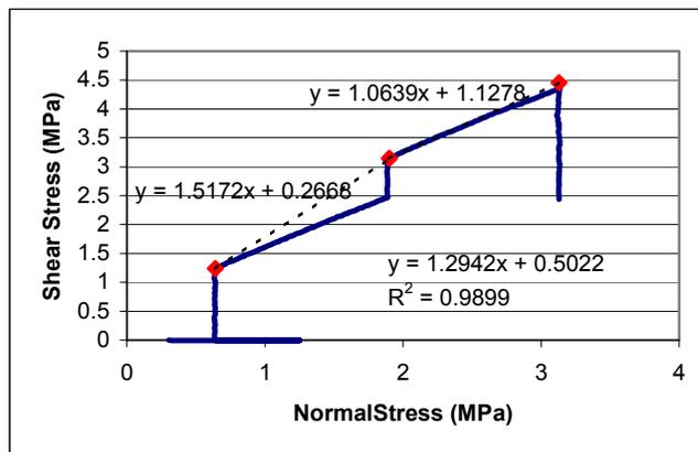
Figure 4. Mohr stress plot for an intact sample sheared perpendicular to the foliation. The friction angle decreases from  $56^\circ$  to  $46^\circ$  while the average value is  $52^\circ$ .
