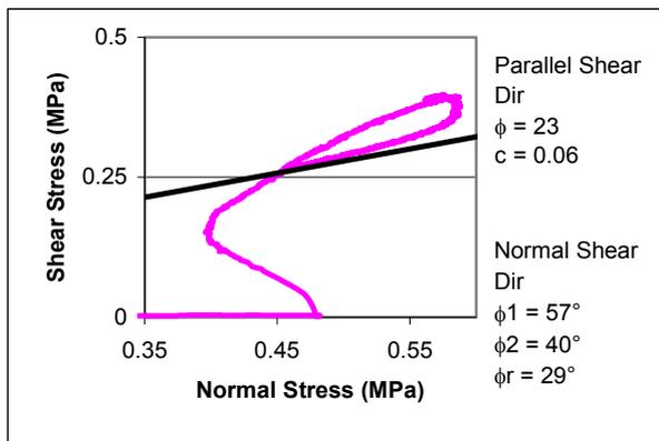
Figure 14. Detail of 10 showing the convergence of the residual line with the failure envelope (straight line) from the test performed parallel to the foliation. The initial contraction of the sample is obvious before dilation begins to occur.
