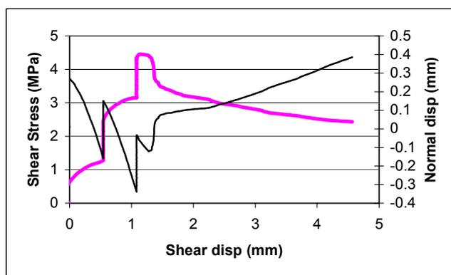
Figure 5. Stress vs. displacement for perpendicular shearing. Note the rapid drop in required shear stress with the localization of shear on a through going shear plane.
