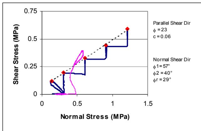
Figure 10. Mohr stress plots for both the CNS and CNL test procedures performed parallel to the foliation (thick line) and the CNS test performed normal to the foliation. Friction angles are displayed on the plot.
