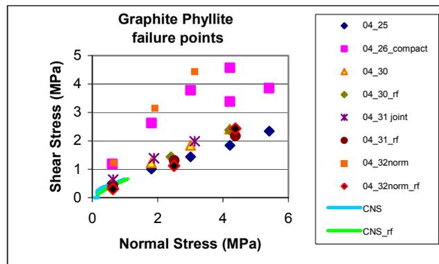
Figure 1. Mohr stress space summary plot of the failure points for the graphite phyllite tests.
