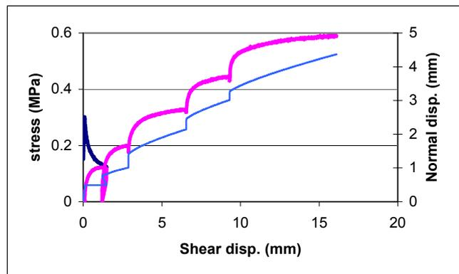
Figure 11. Stress Displacement plot for the parallel sheared sample. The thick lines are the stress lines. The normal stress is only shown for the CNS portion of the line (Drops from 0.3 to 1.5). The dilational characteristics are very similar to the previous test shown in Figure 8.
