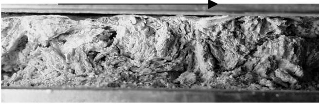
Figure 13. Close up of the shear zone developed during the CNS test perpendicular to the foliation. Sample View is approx. L = 8 cm, H = 1.8 cm. Shear direction was dextral (top to the right). Note the folded mica layers surrounding more competent inclusions indicating a complex deformation band and not simple sliding.
