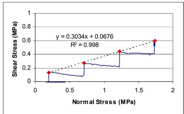
Figure 8. Mohr stress plot for the intact chlorite sample sheared parallel to the foliation. Friction angle is approximately 17°.
