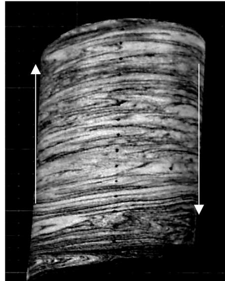
Figure 15. Sample of quartz phyllite (quartz = light, mica layers = dark). Showing the ductile flow structures that dominate these samples. Points are 1 cm intervals. The foliation surfaces are crenulated with consistent properties wavelength 0.5 mm and height approximately 0.05mm.
