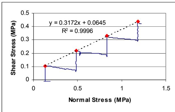
Figure 6. Mohr stress plot for the intact chlorite sample sheared parallel to the foliation. Friction angle is approximately 17.5°.
