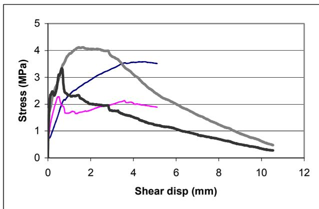
Figure 17. Stress vs. Displacement for the CNS tests parallel to the foliation. Thicker lines represent the stresses for the sample with a high quartz content. The more rounded lines are the normal stresses while the shear stresses show a distinct peak and drop.
