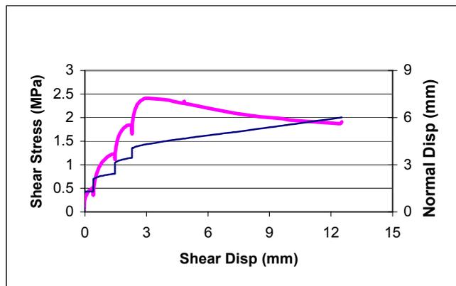
Figure 3. Stress displacement plot for parallel shearing. Thick line is the shear stress and thin line the normal displacement.
