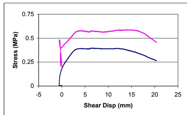
Figure 12. Stress displacement plot for the CNS test with infinite stiffness e.g. zero normal displacement during shear. Once the peak stress is reached the deforms at a constant load before beginning to soften.
