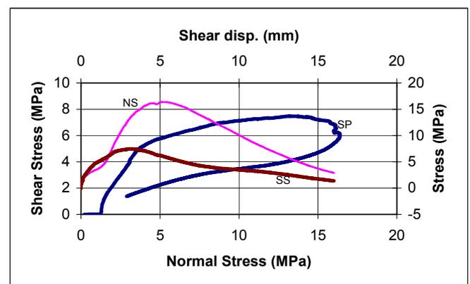
Figure 18. Stress path for the sample sheared perpendicular to the foliation. The stress displacement plots (NS,SS) correspond to the right and upper axis while the stress path (SP) corresponds to the lower and left axis. Note the smooth increase and decrease in the shear and normal stresses.
