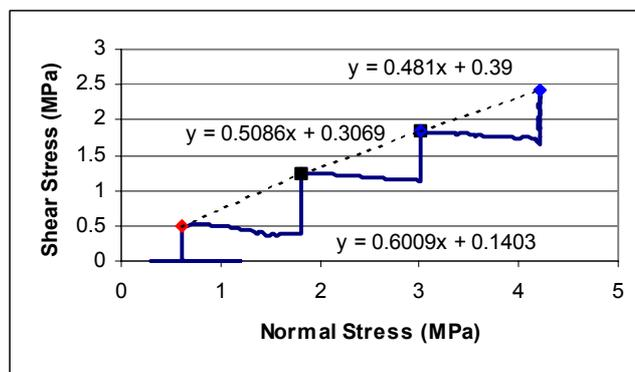
Figure 2. Stress path for an intact sample sheared parallel to the foliation.
