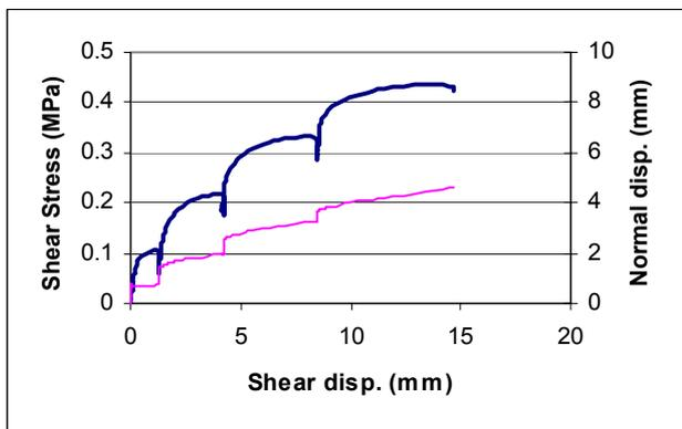
Figure 7. Stress displacement plot for the above test. Thick line is the shear stress while the thin line is the normal displacement.
