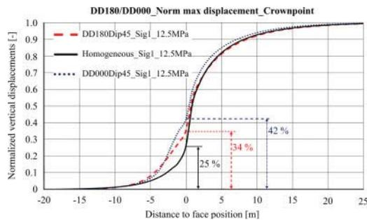
Figure 4. Longitudinal displacement development and influence of the discontinuity orientation.
