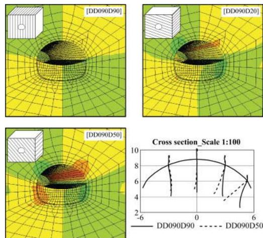
Figure 3. Displacement vector orientation and influence of discontinuity orientation.
