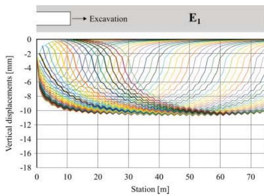
Figure 5. Crown displacement for the tunnel class "BIMRock".
