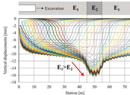
Figure 6. "Monitored" crown displacements.
