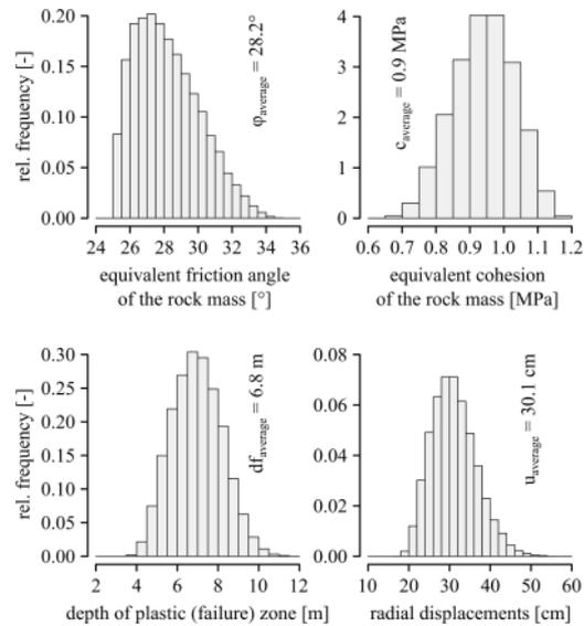
Figure 2. Natural variability of design parameters (upper diagrams) and the effect on results (lower diagrams).
