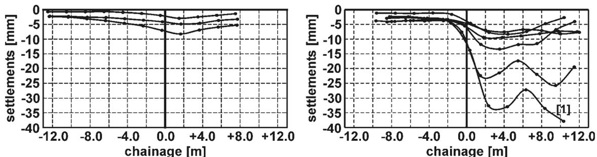
Figure 4. Settlements during the installations of different pipe roofs; left Birgtunnel, right Trojantunnel
