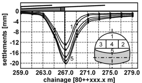
Figure 3. Deflection curves due to one excavation step; left side Birgltunnel, right side Trojanetunnel
