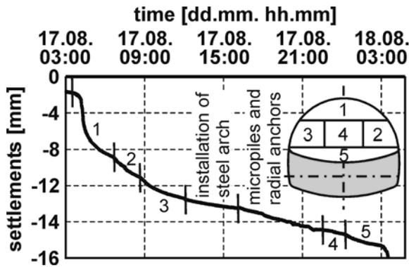
Figure 1. Measured time - settlement line for one excavation step in five phases with support installation
