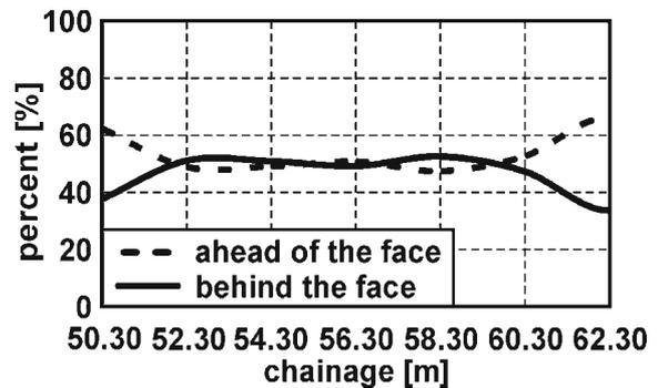
Figure 2. Settlement characteristic in a pipe roof umbrella field (Volkman, 2003)
