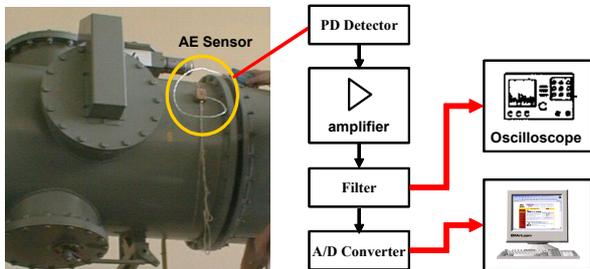
Fig. 4: Acoustic PD detection system
