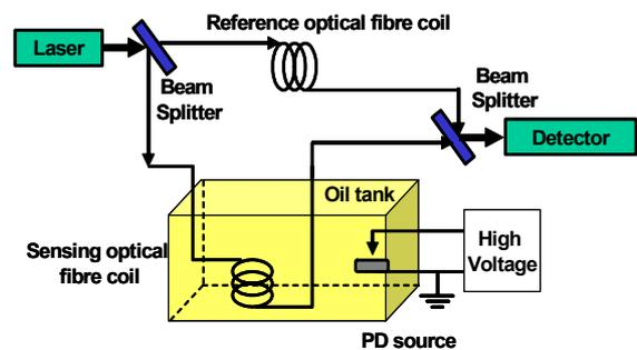
Fig. 5: Experimental setup of the optical interferometric detection of PD [5]
