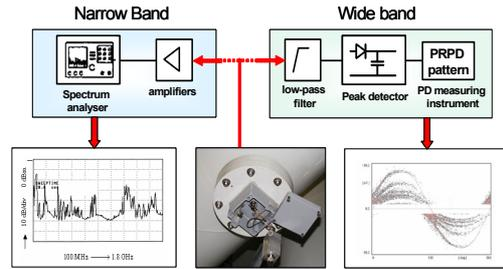
Fig. 1: UHF PD measurement
