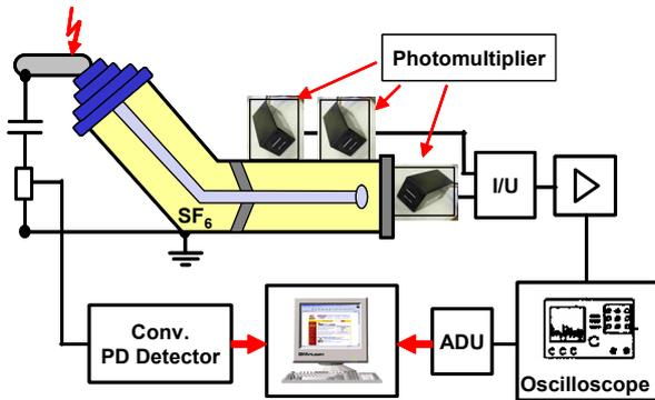
Fig. 7: Test arrangement for optical PD measurement
