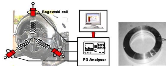
Fig. 2: Measuring for HF PD detection on machines, VHF PD coupler, split ring Rogowski coil [3]
