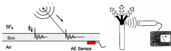
Fig. 3: Principle schematic to the acoustic PD detection
