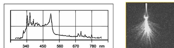
Fig. 6: Spectrum from breakdown arc in SF6 and photo of a discharge [6].
