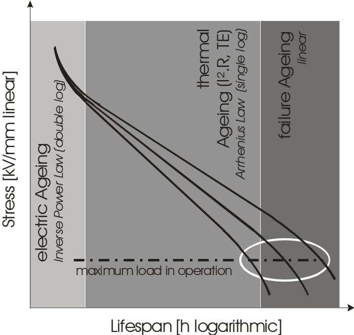
Figure 1: Aging processes, Lifetime in dependence of stress
