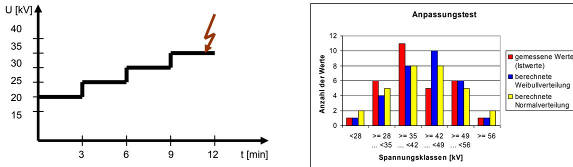
Figure 2: successive discharge test (left) and fitting test (right)
