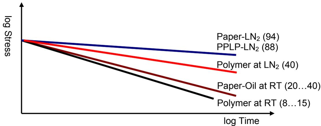
Figure 4: Lifetime curve of different insulation systems, measured and literature of cryogenic and room temperature (RT) insulation systems
