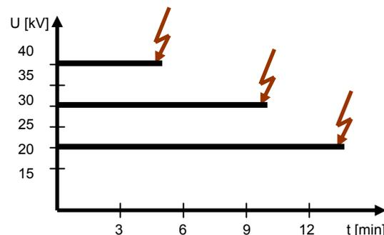
Figure 3: long-time breakdown tests with characteristic loads
