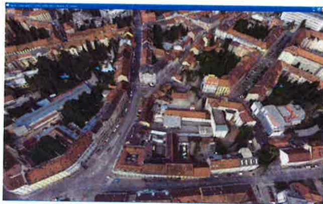
Figure 1: Automatically generated 3D model from a part of Graz. The entire model encompasses 493098 triangles. The image block consists of 155 aerial photographs taken with the UltraCamD camera. Courtesy Microsoft-Virtual Earth, K. Karner.
