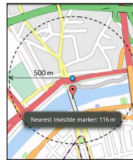
Figure 8: A view on the AARE - blue circle represents the user's GPS location, the red pin is the nearest invisible site which remains inside the discovery radius (500 m)
