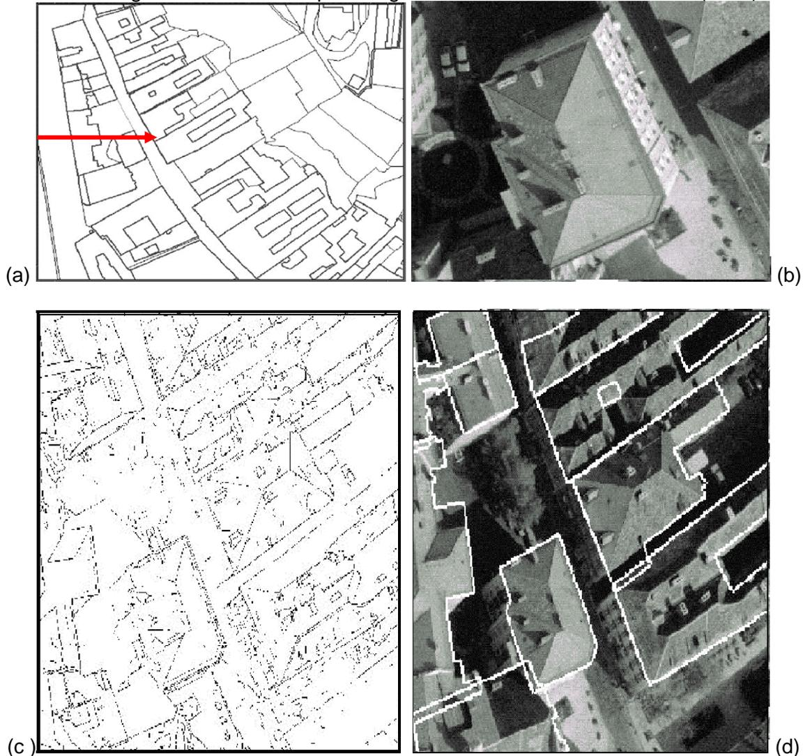
**Figure 13:** A vector data set from a 2D GIS in (a) gets matched with raster data from aerial photos (b) extracting first edges in (c) and then using the technique of “affine matching” (also “chamfer matching”). The match result is shown in (d)
