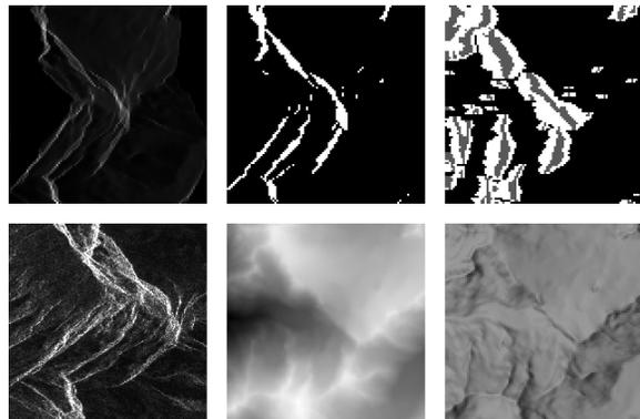
Figure 2: *Result of the simulation process. In the bottom row, from left to right, the original ERS-1 SAR image (©esa), the DEM (higher elevations are displayed as brighter regions), and the backscatter map in DEM geometry. In the top row, the simulated SAR image on the left, the layover map in the geometry of the SAR image in the middle, and the layover map in DEM geometry on the right, where white regions denote passive and gray regions active layover.*
