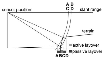
Figure 1: Origin of active and passive layover.
