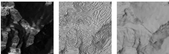
Figure 3: *Simulation of different geocoding processes. From left to right: ordinary geocoding (A), distribution of the intensities according to the number of DEM cells involved (B), and according to the refined method (C) using the backscatter map.*
