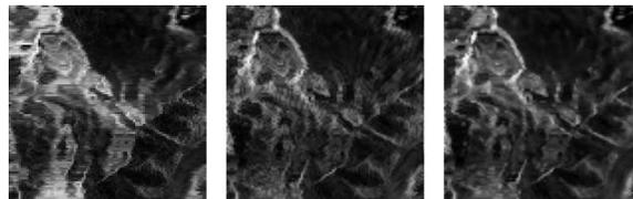
Figure 5: *Geocoding of the original ERS-1 scene. From left to right: usual geocoding (A), distribution of the intensities according to the number of DEM cells involved (B), and according to the refined method (C) using the simulated backscatter map.*
