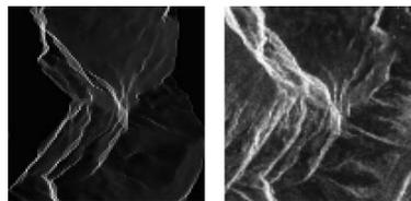
Figure 4: *The original ERS-1 SAR scene after transformation (right) into the geometry of the simulated image (left).*
