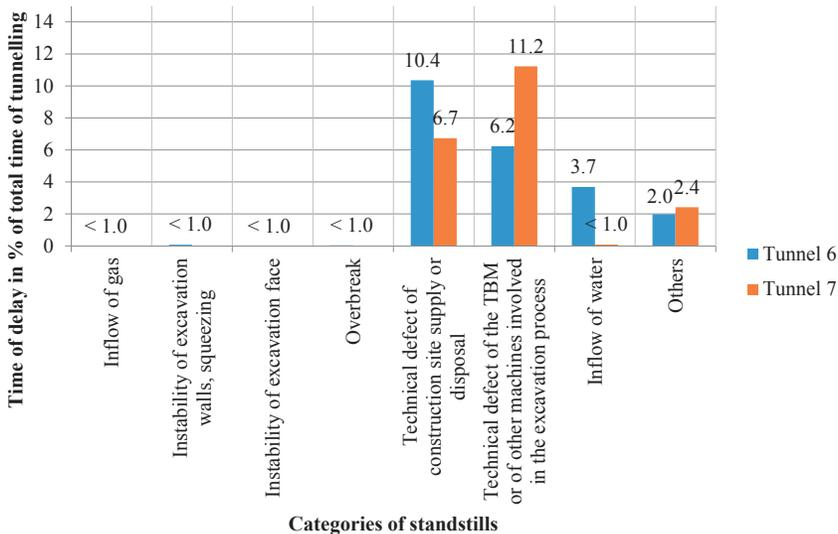
Figure 4. Comparison of unexpected standstills at Tunnel 6 (L1, DSM, D3, O3) and Tunnel 7 (L1, DSM, D3, O3).
