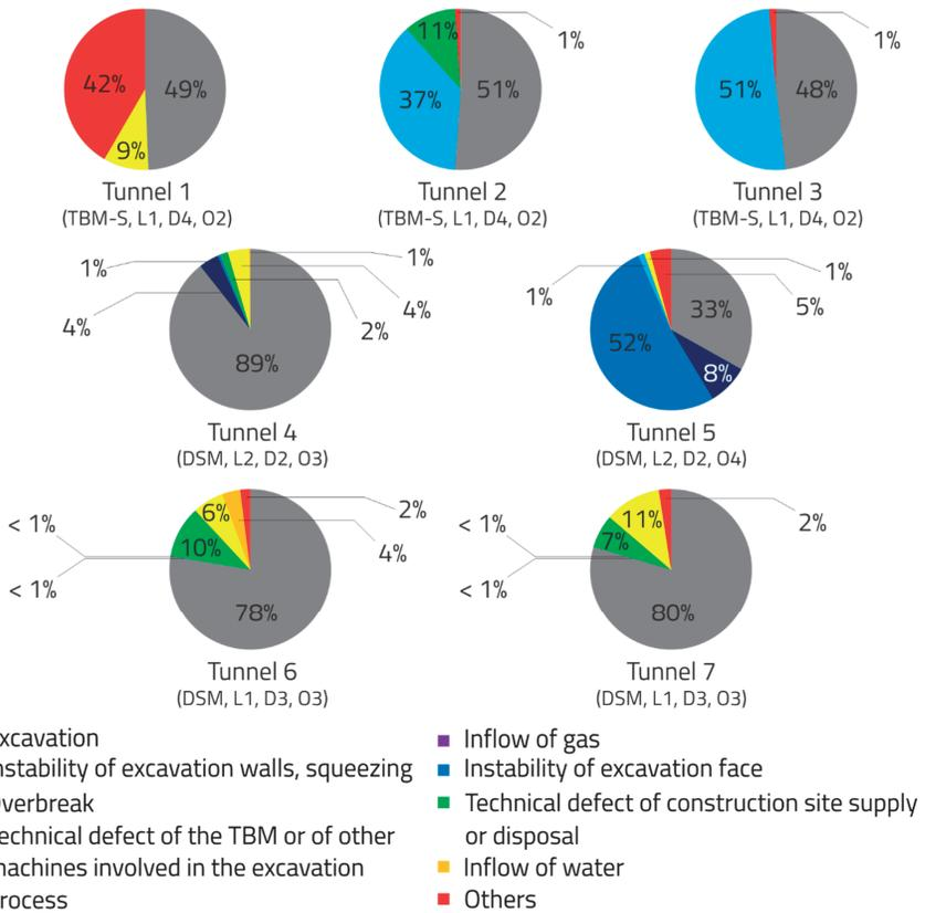
Figure 3. Evaluation of the unexpected standstills of seven projects (maintenance shifts: for Tunnel 1-3 included in “Others”; for Tunnel 4-7 included in “Excavation”).
