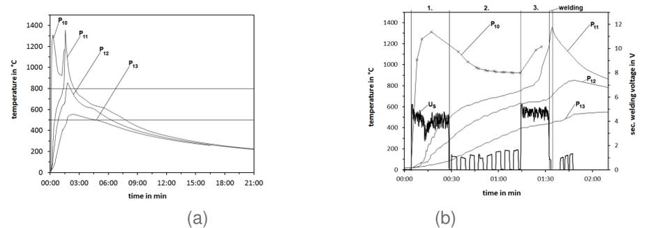
Figure 2:  $T(t)$ -curves at the rail head. (a) ... entire welding sequence. (b) ... heating-phase in detail.  $U_S$  ... secondary welding voltage.
