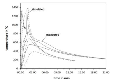
Figure 5: Experimental vs. numerical  $T(t)$ -curves at rail head.
