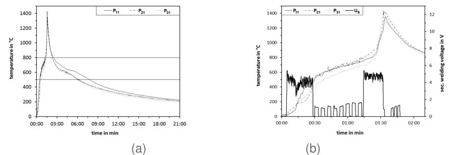
Figure 3:  $T(t)$ -curves closest to the welding face. (a) ... entire welding sequence. (b) ... heating-phase in detail.  $U_S$  ... secondary welding voltage.
