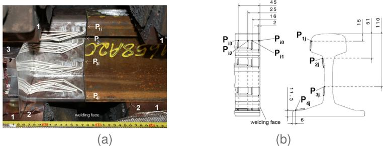
Figure 1: (a) ... instrumented rails. (b) ... measuring positions and labelling. 1 ... welding electrodes 2 ...  $U_S$ -measuring 3 ... protection cover thermocouples.
