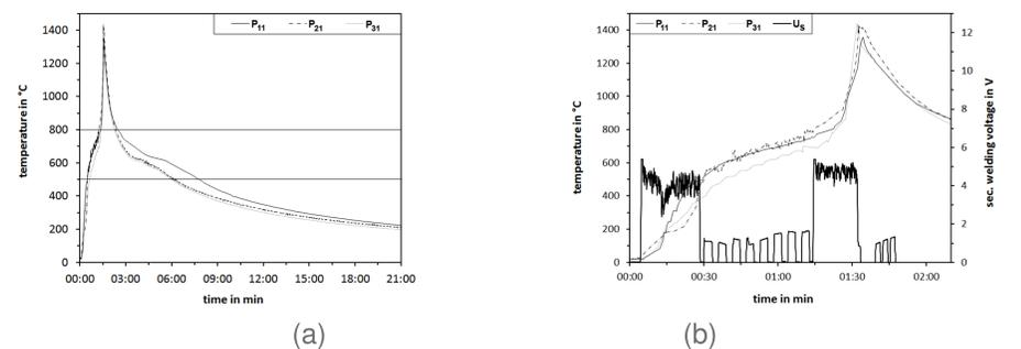
Figure 3:  $T(t)$ -curves closest to the welding face. (a) ... entire welding sequence. (b) ... heating-phase in detail.  $U_S$  ... secondary welding voltage.
