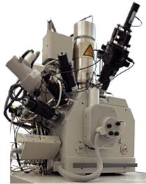
Focused Electron Beam Induced Deposition (FEBID) uses the highly localized decomposition of surface adsorbed precursor molecules via electrons to fabricate functional nanostructures.
