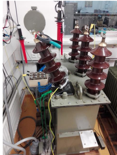
Figure 10: 50 kVA laboratory power transformer
