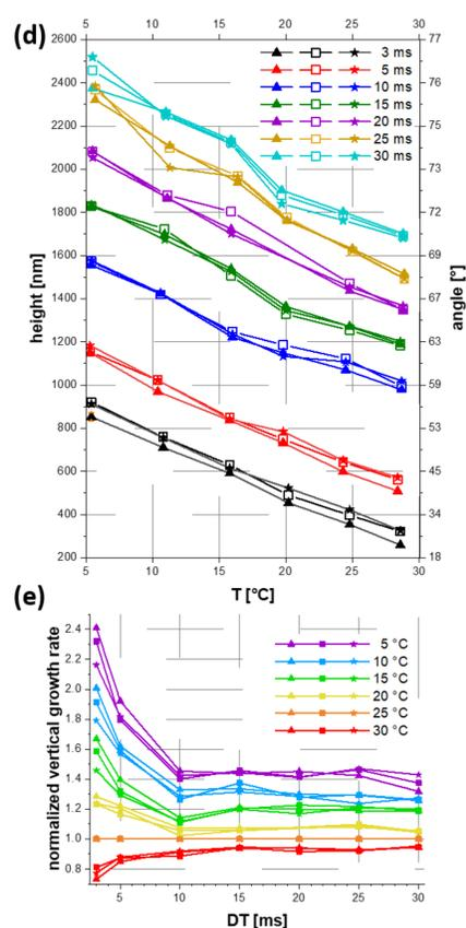
The SEM based growth analysis of tri-, tetra- and pentapods (Fig. 3a-c), fabricated from MeCpPt<sup>(IV)</sup>Me<sub>3</sub> at substrate temperatures T of 5, 10, 15, 20, 25 and 30 °C revealed
