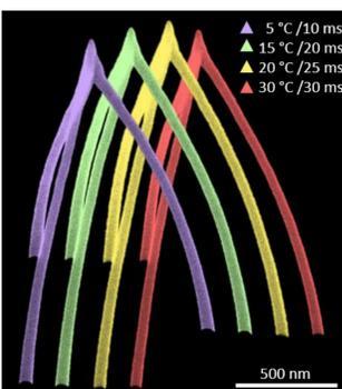
Figure 6: Comparison of tripods with same heights fabricated at different substrate temperatures shows no shape degradation. [3]
