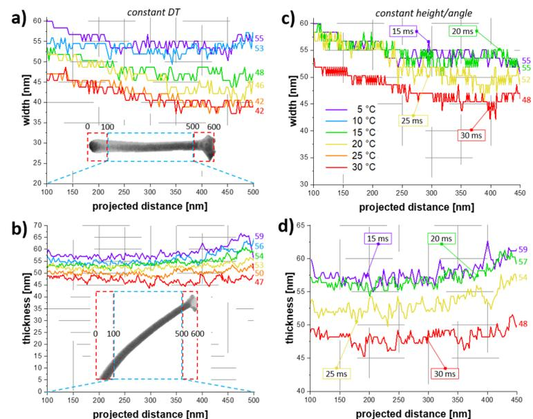
Figure 4: Width and thickness variations along the wires of a tripod. (a,b) compares multipod wires fabricated at 15 ms DT, (c,d) for comparable tall tripods. [3]
