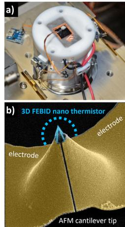
Figure 2: (a) Peltier stage for 3D-FEBID experiments. [3] (b) A FEBID 3D nano-thermistor probe on an electrical accessible self-sensing AFM cantilever as an example of an industrial relevant application. [4]
