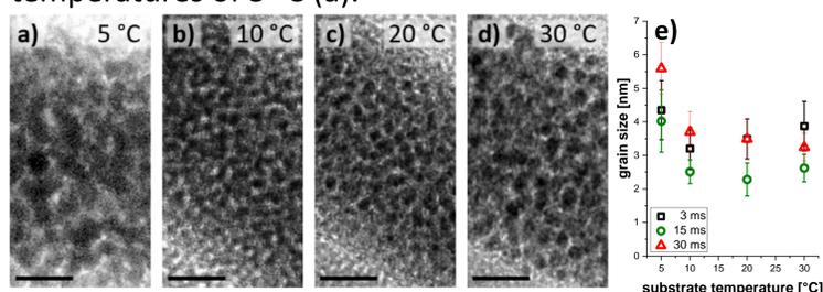
Figure 4: TEM microstructure analysis. TEM images of Pt<sub>x</sub> tetrapod branches fabricated at (a) 5 °C, (b) 10 °C, (c) 20 °C and (d) 30 °C. Scale bars are 10 nm. (e) Mean grain sizes (Feret diameter) for wires fabricated at different substrate temperatures. [3]
