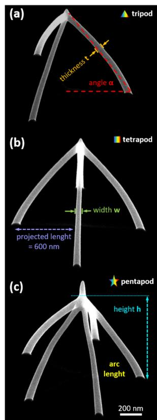
Figure 3: (a-c) PtC multipods (5 keV, 28 pA) on cooled Si-SiO<sub>2</sub> substrate. (d) Structure heights as a function of the substrate temperature and (e) vertical growth rates. [3]
