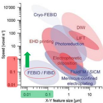
Figure 1: Comparison of 3D-nanoprinting techniques [1]
