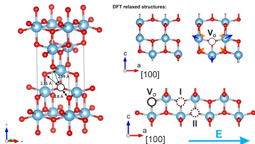
Figure 1: Structure of TiO<sub>2</sub> anatase and VO arrangement. Applied *E* field vector parallel to [100] orientation.
