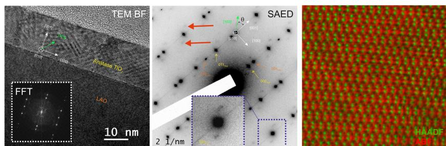
Figure 2: Structure of TiO<sub>2</sub> anatase and VO arrangement
