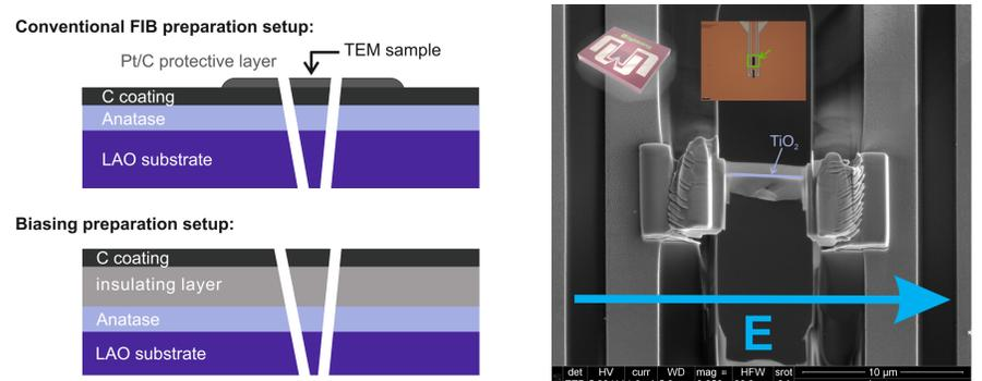
Figure 3: TEM biasing sample preparation procedure
