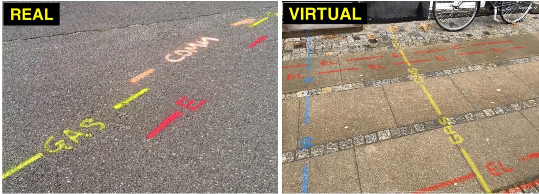
**Figure 1.2: Virtual Spray marking:** An AR application for automated spray paint marking of SUE utilities. Left image show real spray markings on the surface, right image in contrast show the virtual spray markings. Realism of visualization can be achieved by overlay blending in combination with accurate 3D LIDAR reconstruction of the environment. *Images from our previous work [4].*
