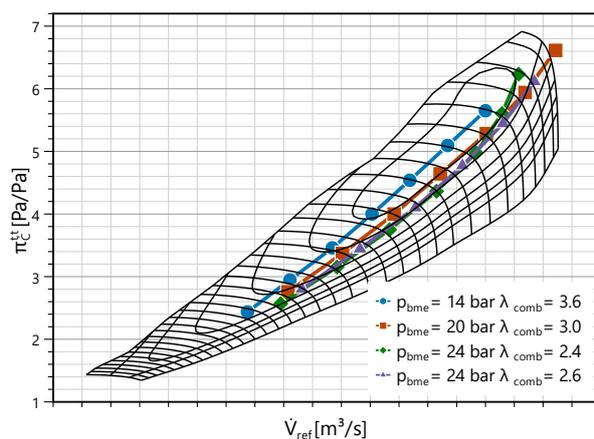
Figure 17. Engine operating lines on compressor map for selected cases
