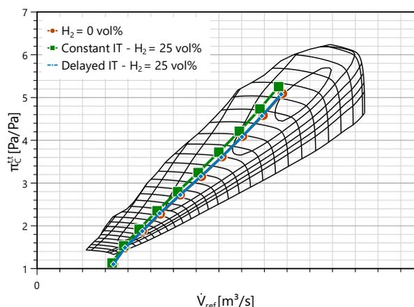
Figure 11. Influence of a delayed ignition timing on the position of the engine operating line on the compressor map
