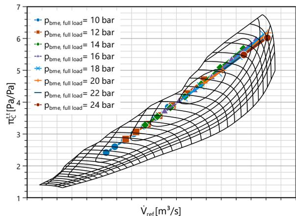
Figure 18. Operating points for various mean effective pressures and excess air ratios compared to typical compressor map of A200-H [13]
