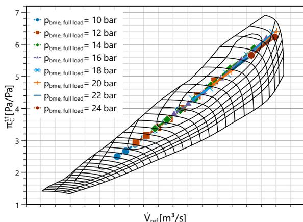
Figure 13. Operating points for various mean effective pressures and excess air ratios compared to typical compressor map of A200-H [13]
