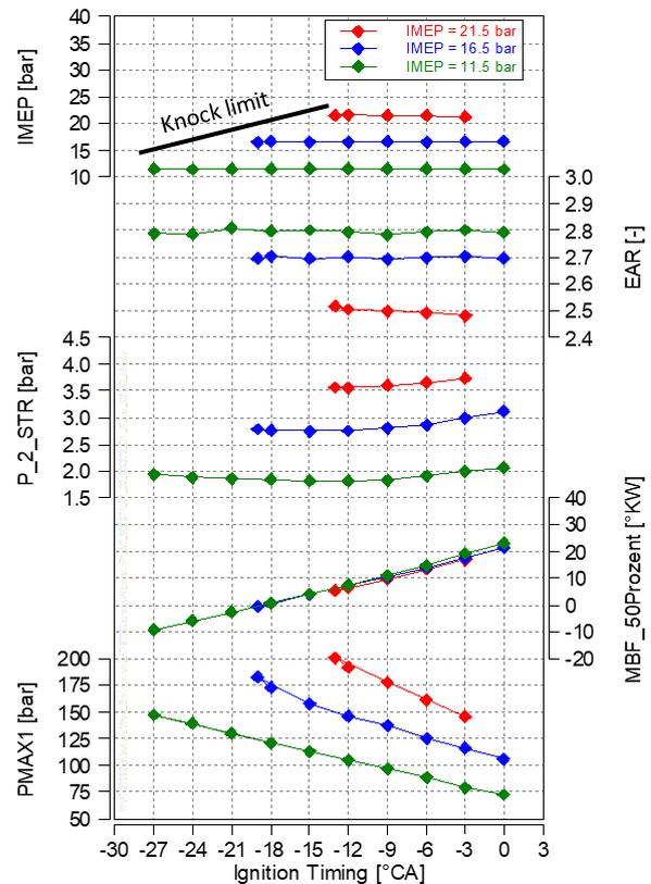
Figure 7. SCE performance parameters for hydrogen operation at various IMEP
