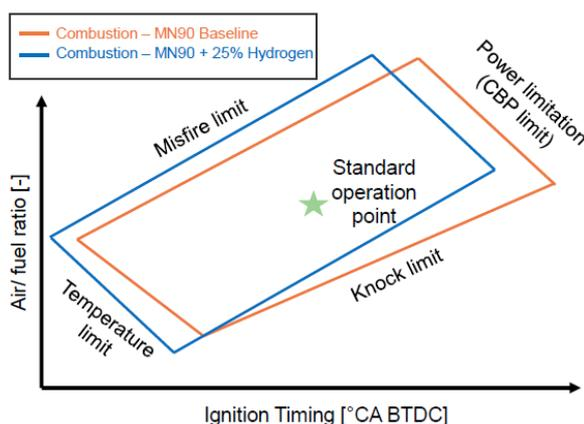
Figure 4. Operating window for natural gas operation and operation with 25 % hydrogen blending at full load
