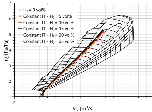
Figure 10. Positions of engine operating lines on the compressor map for various hydrogen admixture rates to natural gas
