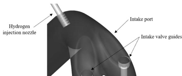
Figure 6. Position of the hydrogen injection nozzle in the intake port (Type 6)
