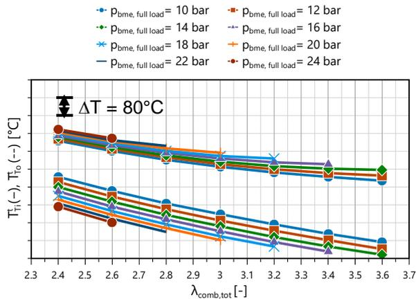
Figure 16. Temperatures at turbine inlet and outlet for various mean effective pressures and excess air ratios
