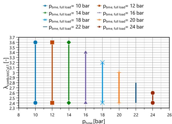
Figure 14. Feasible excess air ratios at various mean effective pressures
