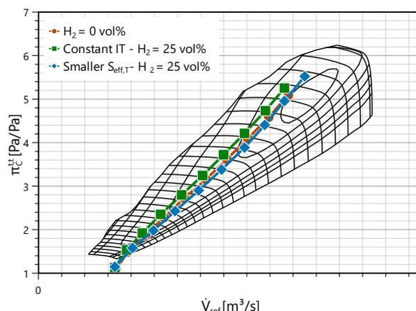
Figure 12. Influence of a modified turbocharger matching on the position of the engine operating line on the compressor map
