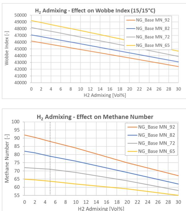
Figure 3. Wobbe Index (WI) and Methane Number (MN) change depending on H<sub>2</sub> content in pipeline gas [5]
