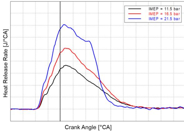
Figure 8. Heat release rates for pure hydrogen operation for different indicated mean effective pressures
