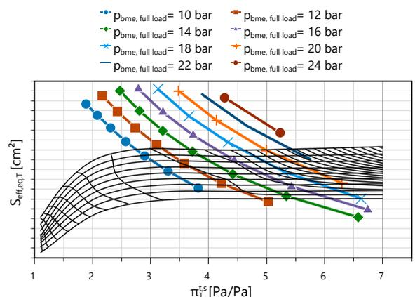
Figure 15. Operating points for various mean effective pressures and excess air ratios compared to nozzle rings of smallest A200-H [13] turbine trim
