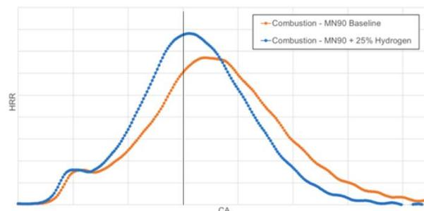
Figure 5. Heat release rate for natural gas operation (orange) and 25 % hydrogen blending to natural gas (blue)
