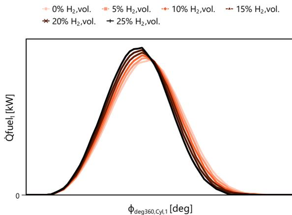
Figure 9. Heat release rates for various hydrogen admixture rates to natural gas
