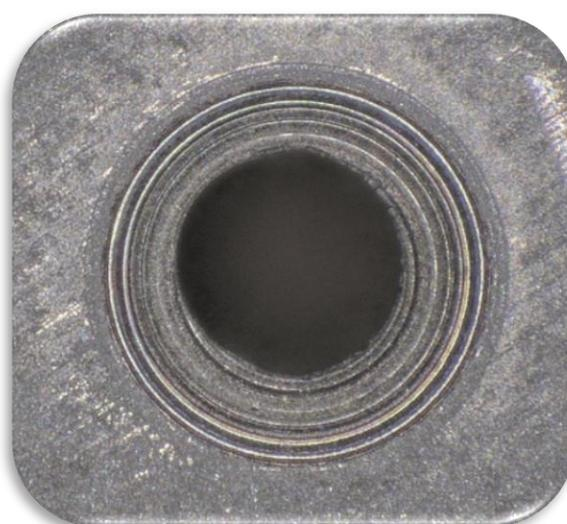
Figure 3: Hard metal control valve seat conditions after operation with methanol and 10 bar backpressure.
