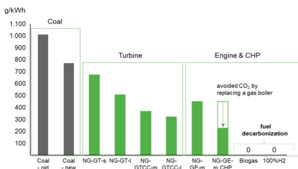
Figure 3. CO<sub>2</sub> intensity of different technologies
