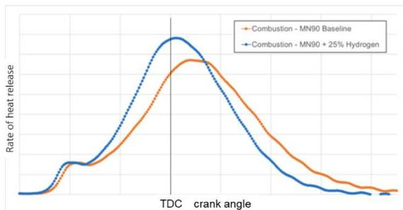
Figure 6. Heat release rate for natural gas vs. hydrogen combustion
