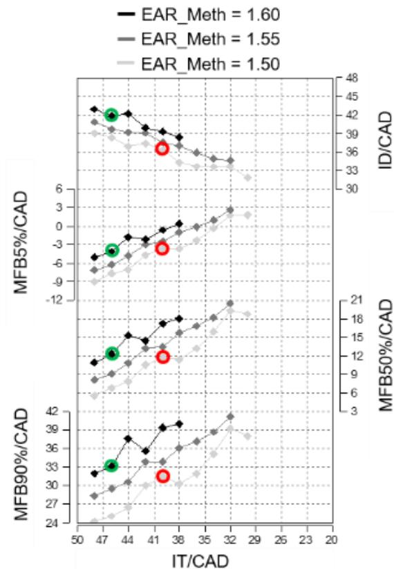
Figure 20. Combustion variability for methanol operation in an open chamber configuration
