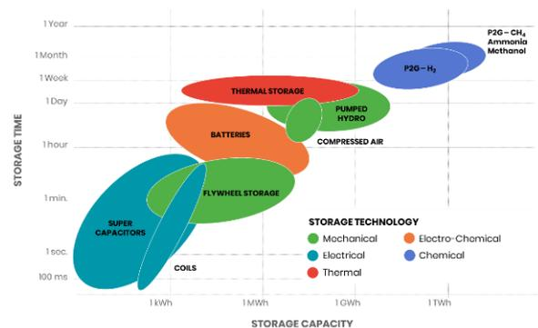
Figure 2. Energy storage options capacity vs. duration
