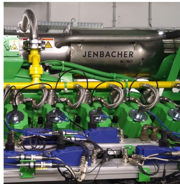
Figure 11. INNIO's Jenbacher hydrogen engine
