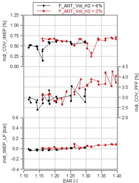
Figure 15. Selected performance parameters for ammonia/hydrogen combustion @ 23 bar IMEP
