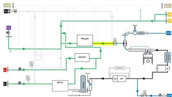
Figure 13. Test infrastructure for ammonia engine operation
