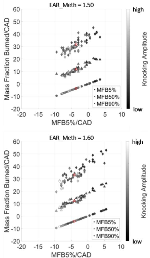
Figure 21. Combustion variability for methanol operation in an open chamber configuration
