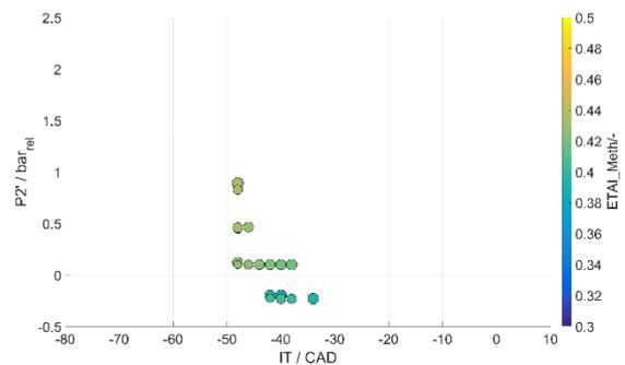
Figure 19. Operating window for methanol fuel combustion concept
