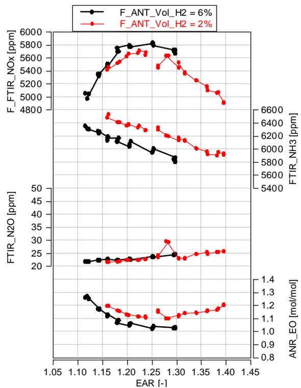
Figure 16. Selected engine-out emissions for ammonia/hydrogen combustion @ 23 bar IMEP
