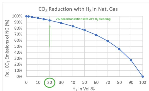
Figure 4. CO<sub>2</sub> reduction with H<sub>2</sub> in natural gas
