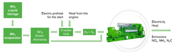
Figure 18. NH3 supply and cracker for a large engine
