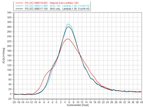
Figure 17. Rate of heat release with different fuel types
