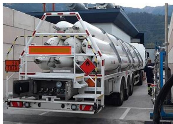
Figure 5. Hydrogen trailer for engine testing
