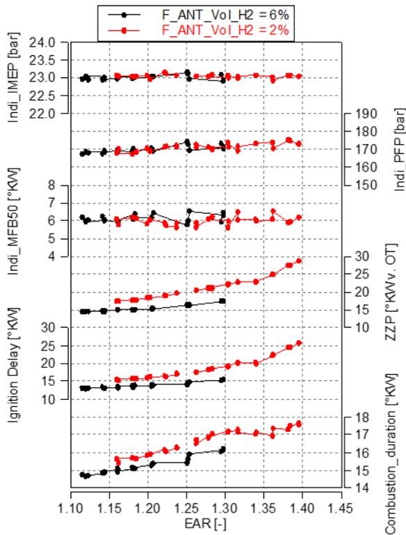
Figure 14. Selected measurement results for ammonia/hydrogen combustion @ 23 bar IMEP
