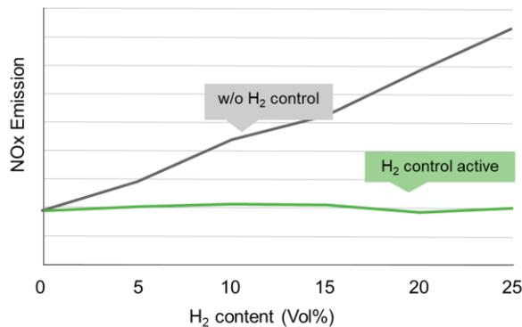
Figure 7. NOx emission with/without active H2 control
