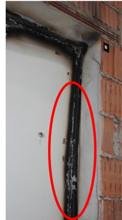
**Figure 21.** Observed gap formation during the fire resistance test at the upper edge of the door (left) and burning marks above the door lock after the test (right)
