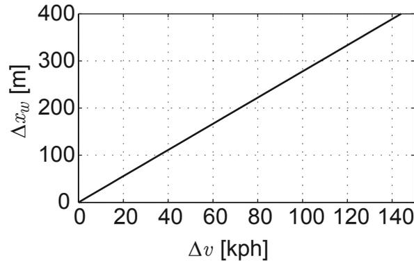
Figure 8.11.: Collision warning distance  $\Delta x_w$  of the  $TTC_{10}$  FCWS model
