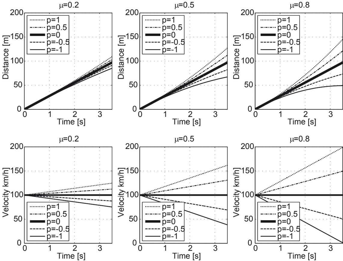
Figure 8.6.: Variation in stopping distance and collision velocity
