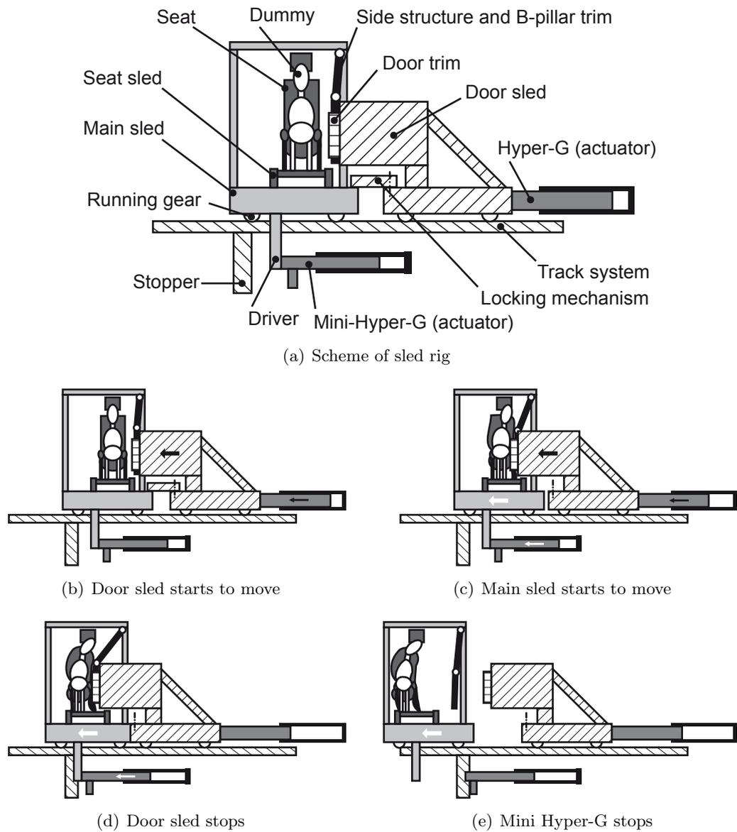
Figure 6.11.: Operating principle of the sled rig
