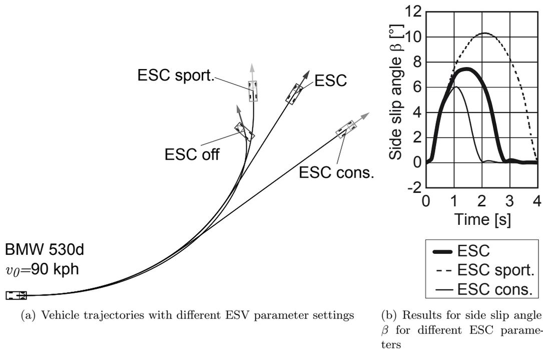
Figure 7.7.: Results for different ESC parameter settings with vehicle BMW 530d, pulse-steer-input manoeuvre with  $v_0 = 90$  kph
