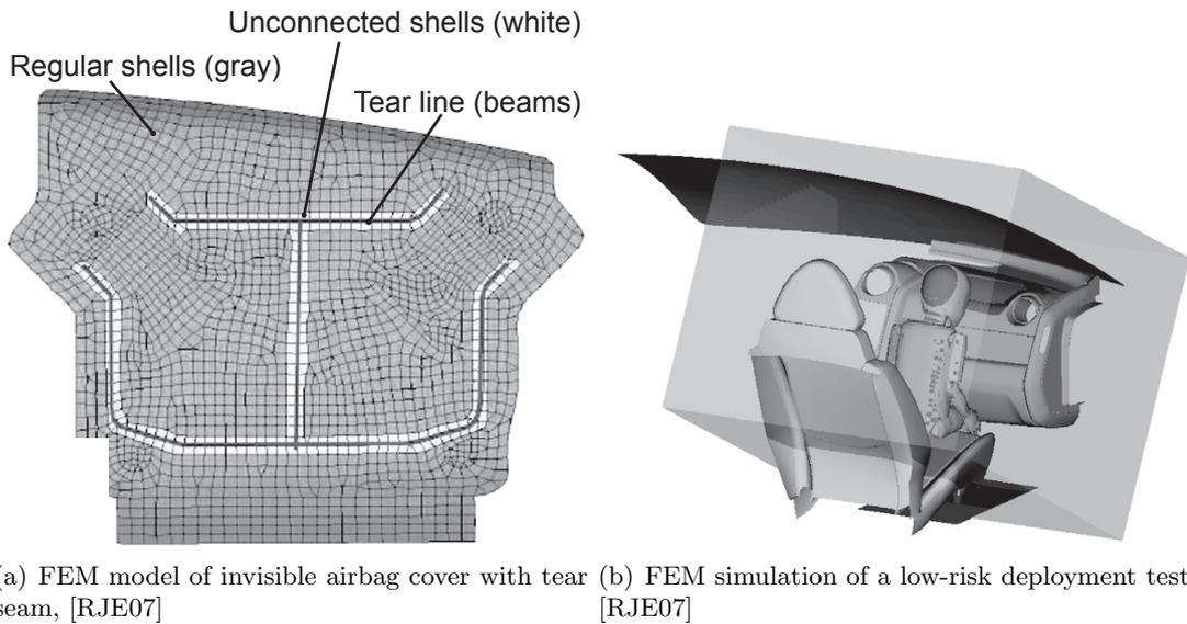
Figure 6.8.: Simulation of low-risk airbag deployment
