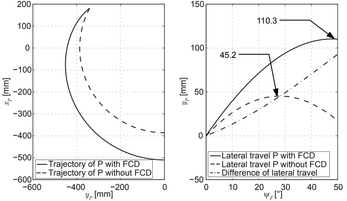
Figure 6.6.: Kinematics of point P with and without the Flexible Collision Deflector
