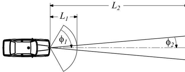
Figure 7.9.: Radar-based environment recognising system for Predictive Brake Assist [ETRH09]
