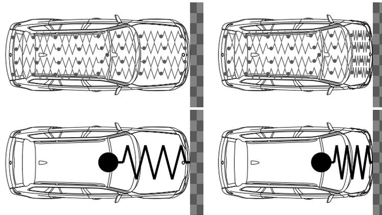
Figure 8.33.: Comparison of single mass and multi mass model
