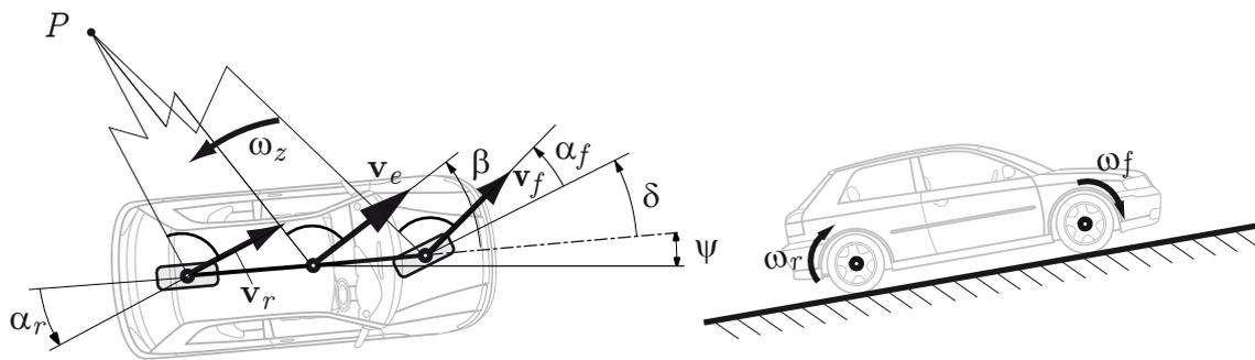
Figure 8.26.: Kinematic quantities for single-track model
