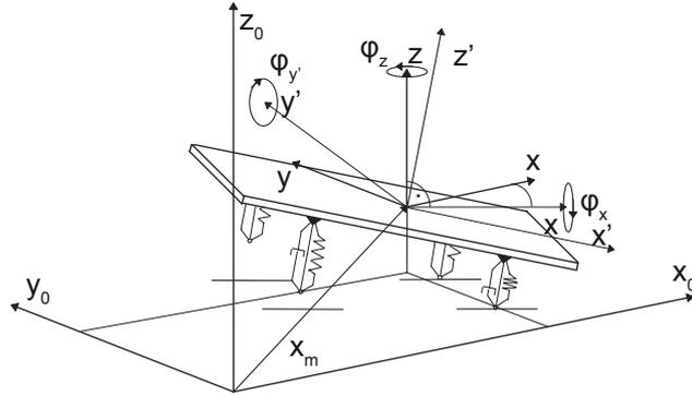
Figure 7.2.: Modelling of vehicles in PC-crash [Ste09a]
