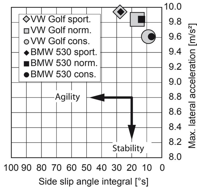
Figure 7.8.: Assessment of different ESC parameter settings
