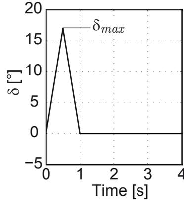
Figure 7.6.: Steering angle  $\delta$  vs. time in pulse-steer-input driving test
