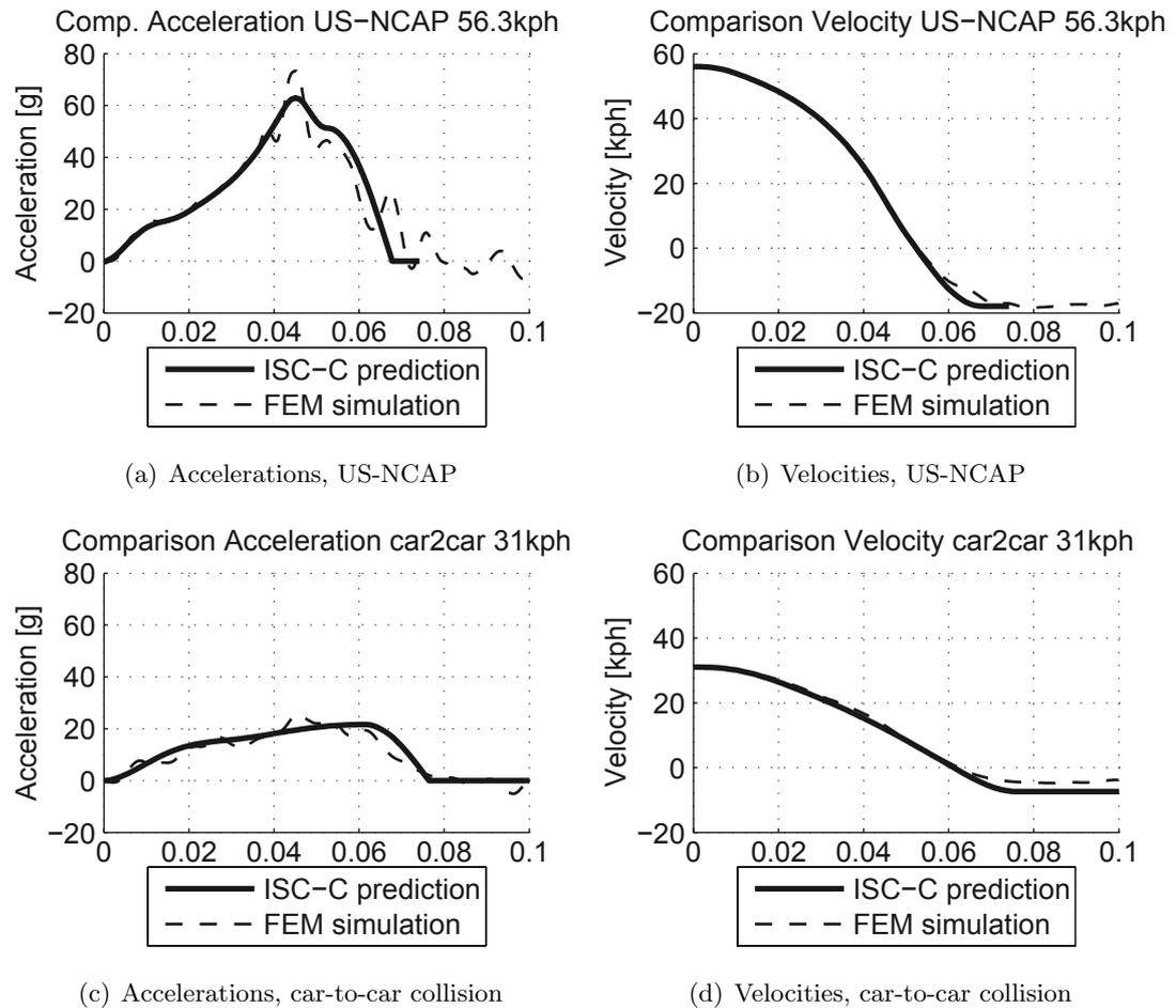
Figure 8.36.: Verification of ISC-C acceleration prediction, [WEHC09]
