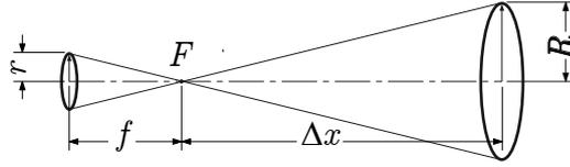
Figure 8.16.: Scheme of an object projected on the human retina
