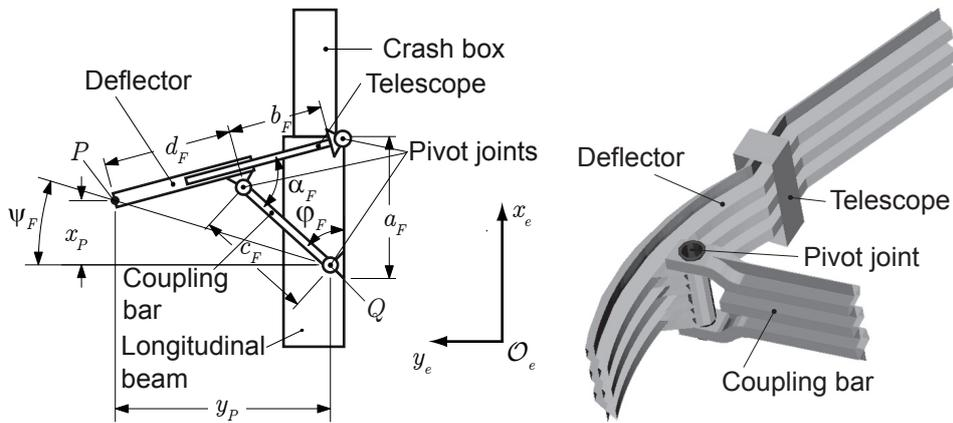
(a) Scheme of Flexible Collision Deflector (FCD), [SE05]      (b) Application of FCD in vehicle, [ESW<sup>+</sup>06]
