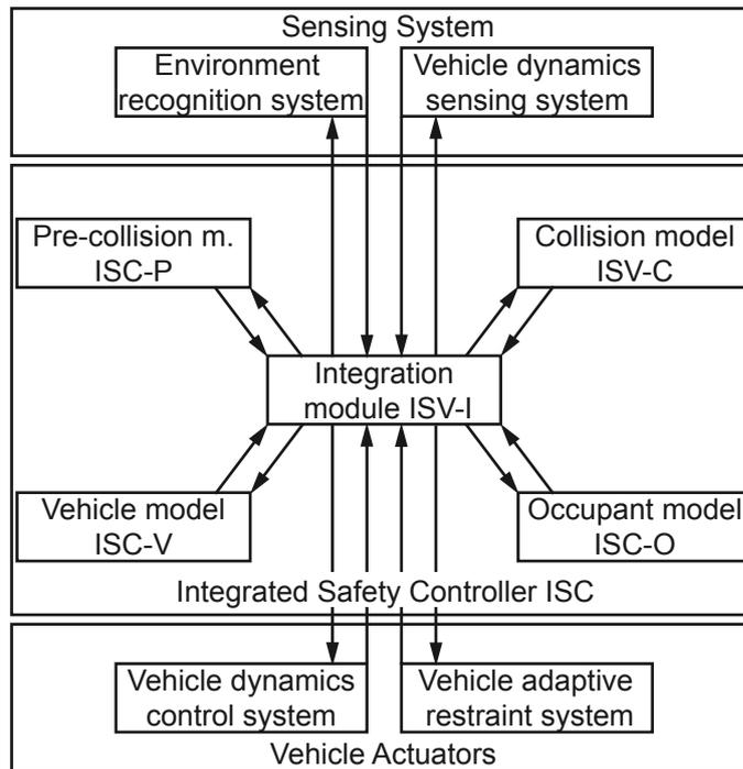
Figure 8.2.: System architecture of the Integrated Safety Controller ISC
