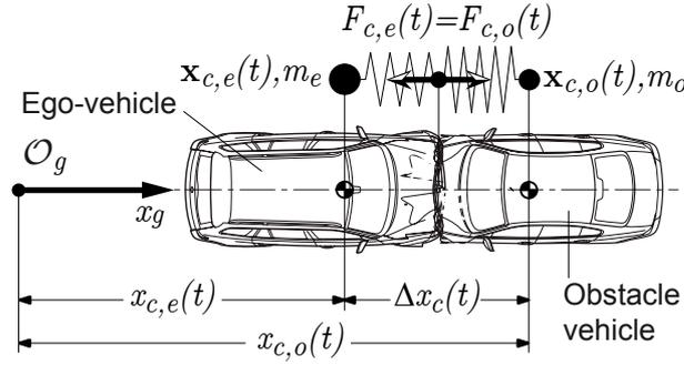
Figure 8.30.: Sketch of combined virtual force concept
