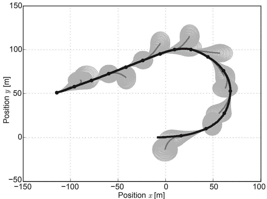
Figure 8.21.: Trajectory prediction with linear KF model, adapted from [Pij08, Pue09] The thick black line represents the vehicle trajectory obtained by simulation. The grey lines are predictions by the linear KF model. Each prediction starts at a time step represented by the black dot. The ellipsoids depict possible locations of the vehicle, depending on driver control input.
