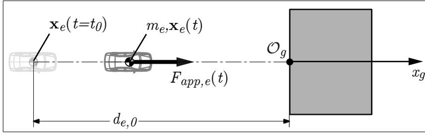
Figure 8.5.: Single mass point collision prediction model for stationary objects
