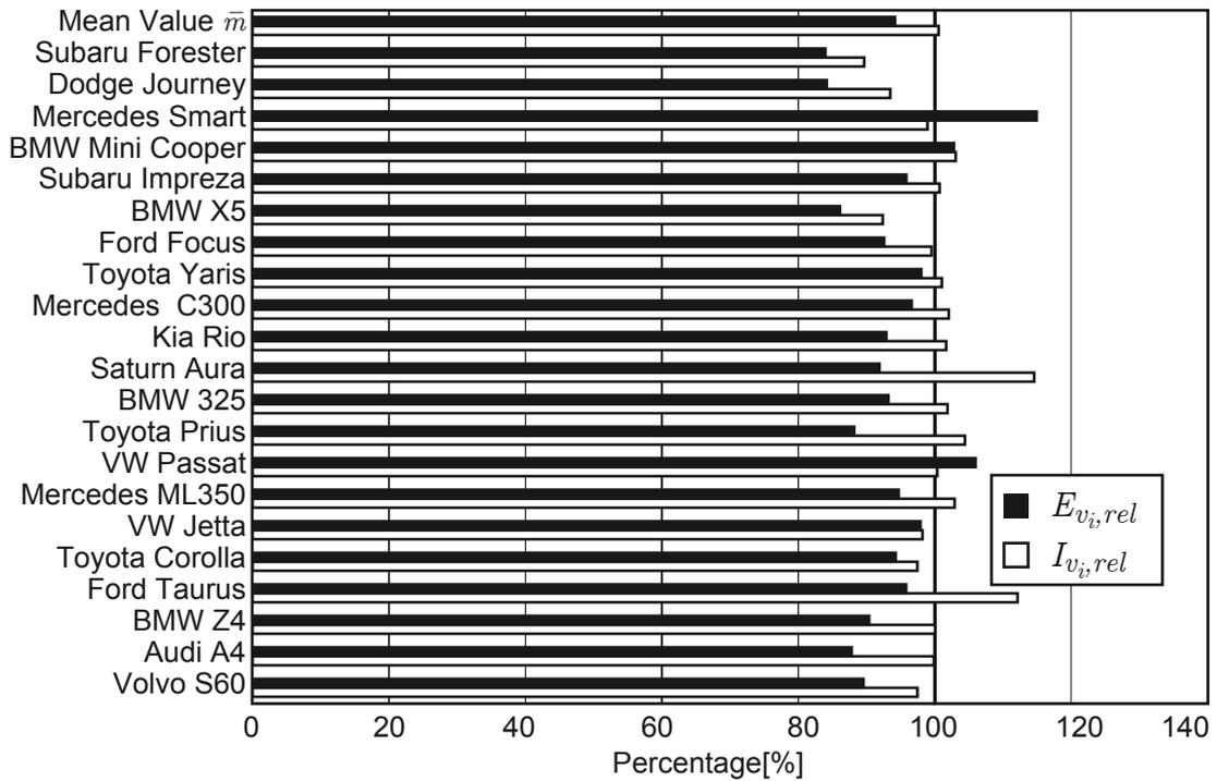
Figure 8.34.: Comparison of impulse and energy between vehicle and rigid barrier measurements
