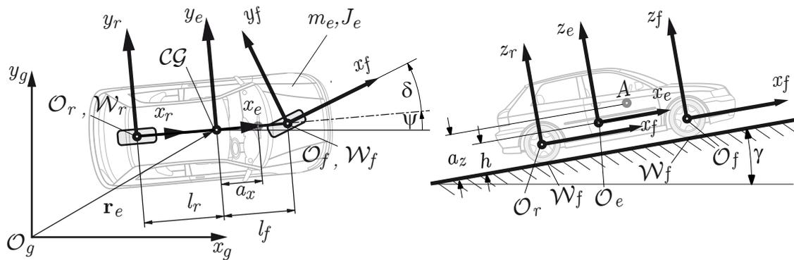
Figure 8.25.: Coordinate systems for single-track model
