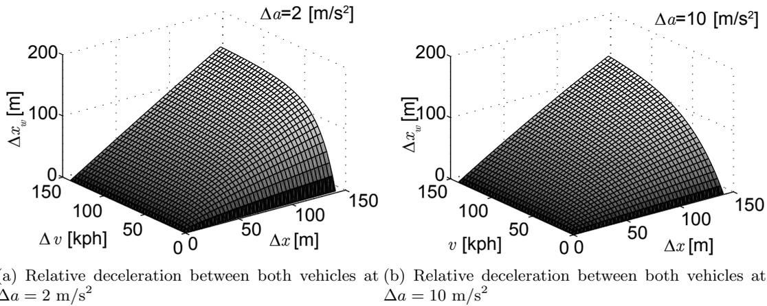
Figure 8.14.: Warning distance in the case of a moving preceding vehicle, algorithm by Barber et al.
