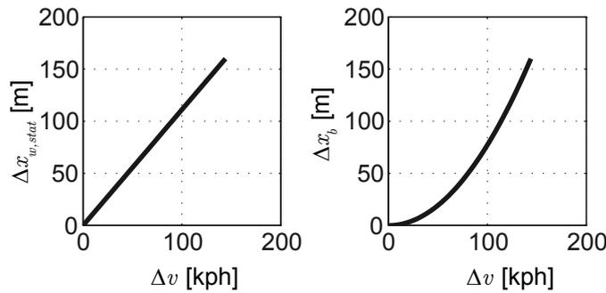
Figure 8.15.: Warning/Braking distance in the case of a stationary preceding vehicle, algorithm by Barber et al.
