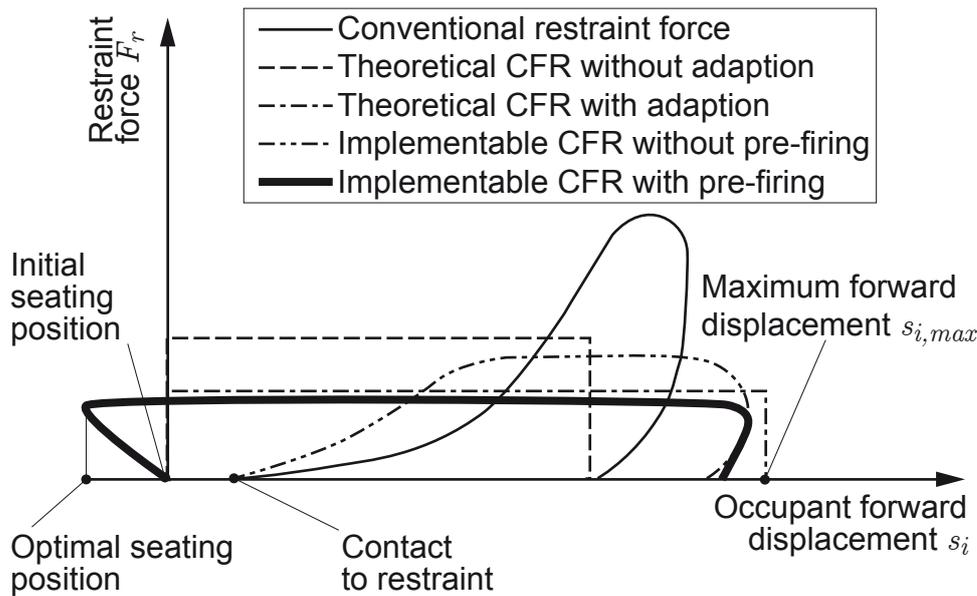
Figure 8.37.: Qualitative illustration of restraint forces, adapted from [Ste09b]
