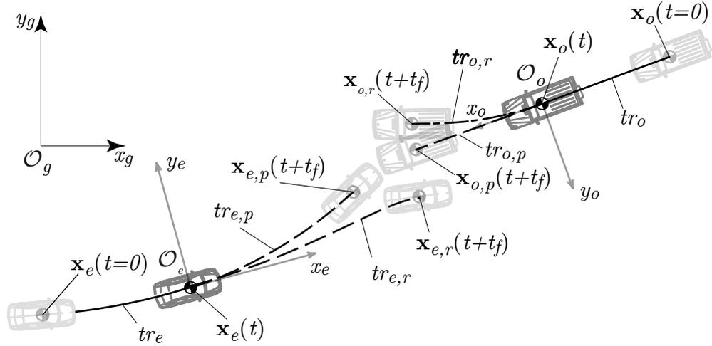
Figure 8.18.: Illustration of collision prediction
