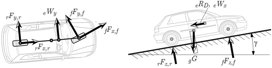
Figure 8.27.: Kinetic quantities for single-track model
