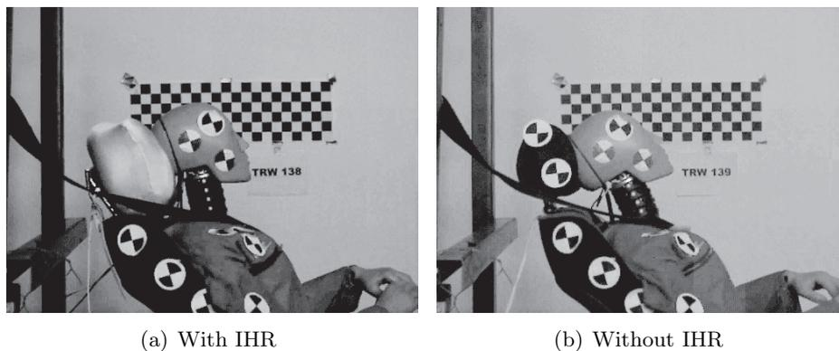
Figure 6.17.: Comparison of dummy kinematics with and without a proactive head restraint.
