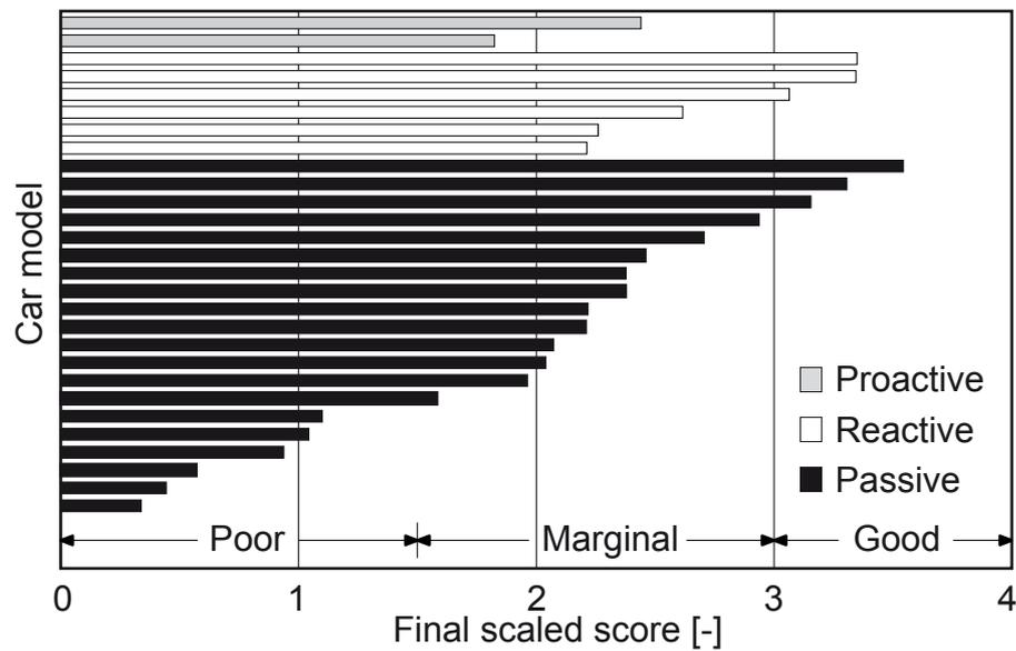
Figure 6.16.: Results of recent EURO-NCAP whiplash seat tests, adapted from [vREA<sup>+</sup>09]
