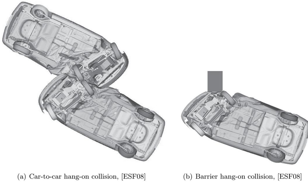
Figure 6.4.: Comparison of hang-on collisions (FEM simulation)
