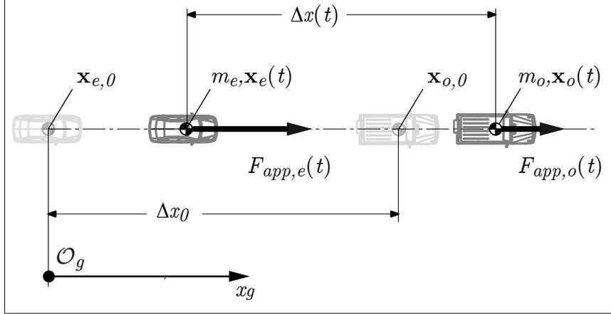
Figure 8.8.: Single mass point collision prediction model, moving preceding vehicle
