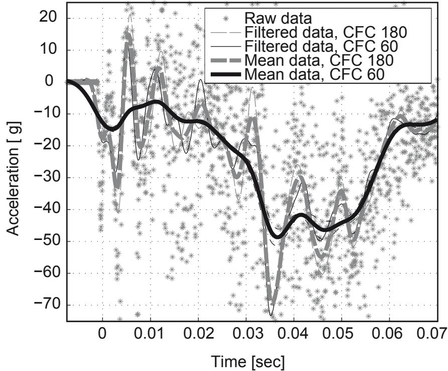
Figure 8.31.: Example of acceleration data processing, [Wal09]
