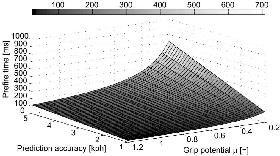
Figure 8.7.: Pre-fire times calculated by the single mass point collision prediction model. The theoretical pre-fire time as calculated by the single mass point collision prediction model. Depending on the accuracy of the prediction of the collision velocity and the adhesion potential between road and tyre, the values vary from 25 to about 1000ms, Tab. 8.1
