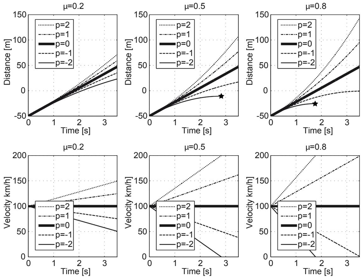
Figure 8.9.: Variations in relative distance and velocity between ego and moving preceding vehicle
