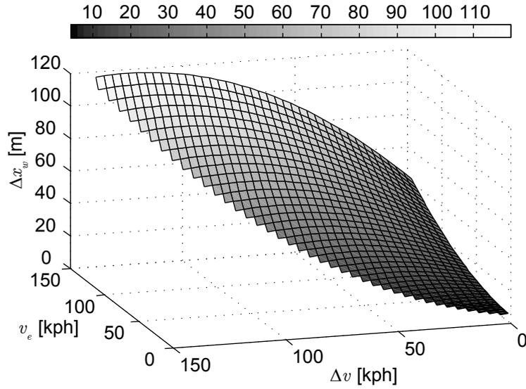
Figure 8.12.: Warning/Braking  $\Delta x_w$  distance of algorithm by Doi et al.
