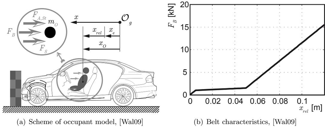
Figure 8.38.: Occupant model ISC-O
