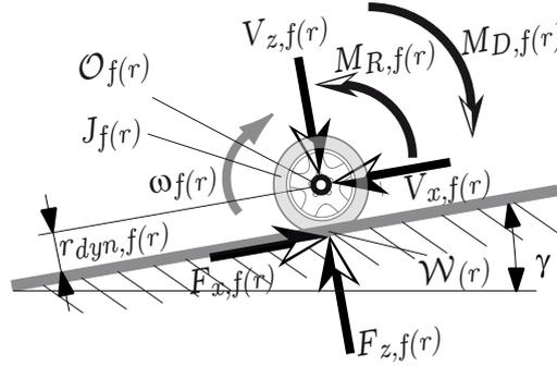
Figure 8.28.: Kinetic quantities for front (f) and rear tyre (r)
