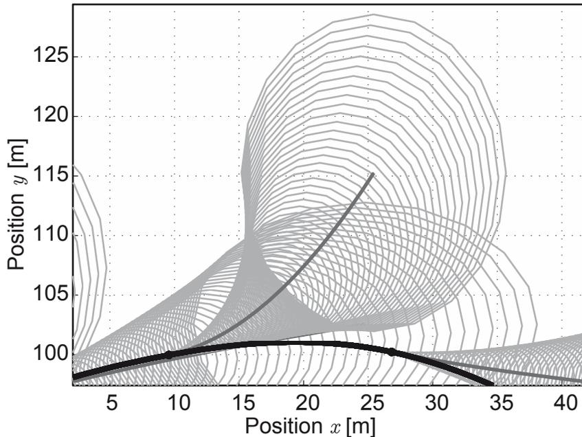
Figure 8.22.: Failure of prediction with linear KF model model
