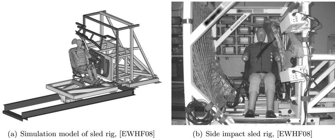
Figure 6.12.: Verification on system level by sled rig
