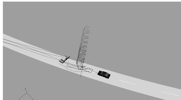
(b)  $t=1.5$  s, skidding of vehicle 1 due to  $\mu_{split}$  braking
