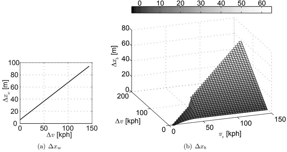
Figure 8.13.: Warning and braking  $\Delta x_w$ ,  $\Delta x_b$  distance of algorithm by Fujita et al. The left figure depicts  $\Delta x_w = f(\Delta v)$ ; note the simple linear relationship. The right figure depicts the autonomous braking intervention. Braking is applied at  $\Delta x_b = f(\Delta v, v_e)$
