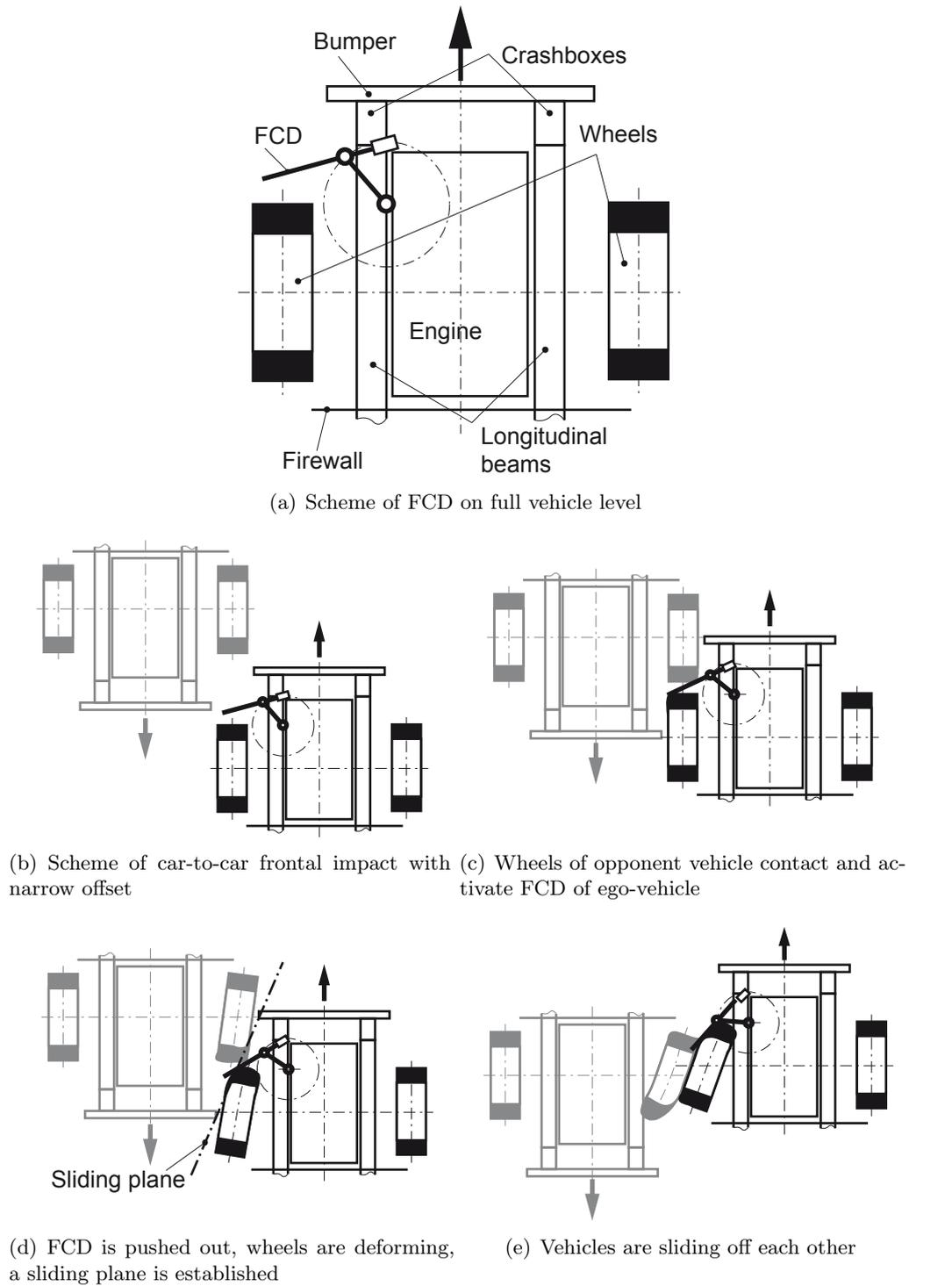
Figure 6.7.: Operating principle of Flexible Collision Deflector, adapted from [SE05]
