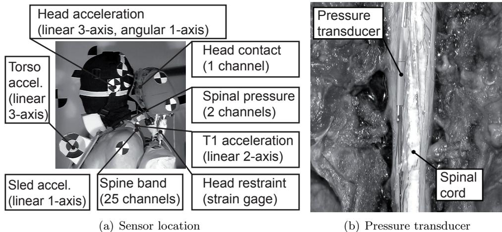
Figure 6.14.: Instrumentation of PMHS tests [EDS<sup>+</sup>00]
