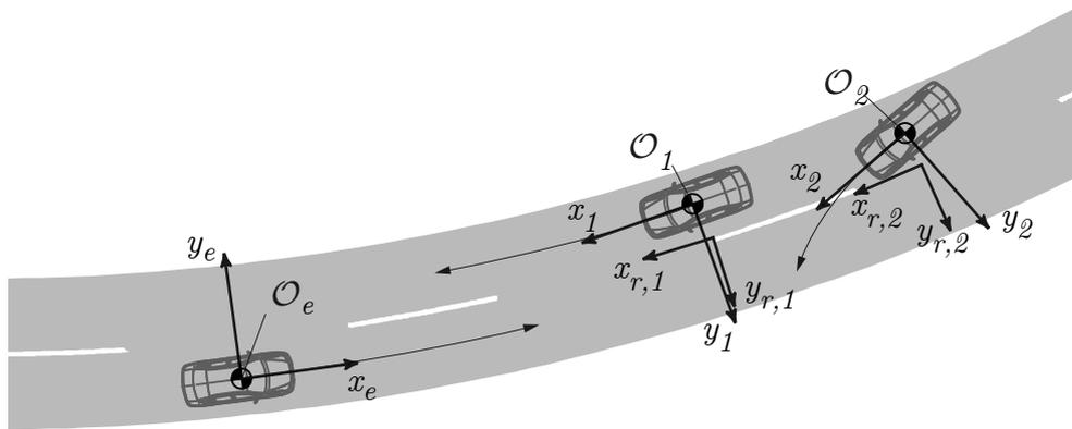
Figure 8.19.: Estimation of vehicle trajectories, according to [BSW07]
