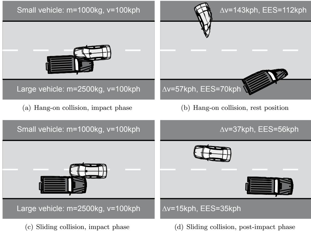
Figure 6.3.: Example of a frontal impact with narrow lateral offset, adapted from [WFBS01]
