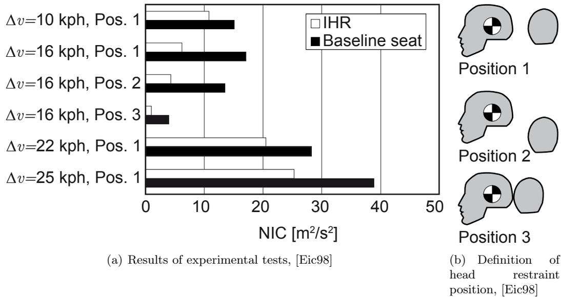
Figure 6.18.: Reduction of  $NIC$  by Inflatable Head Restraint (IHR)
