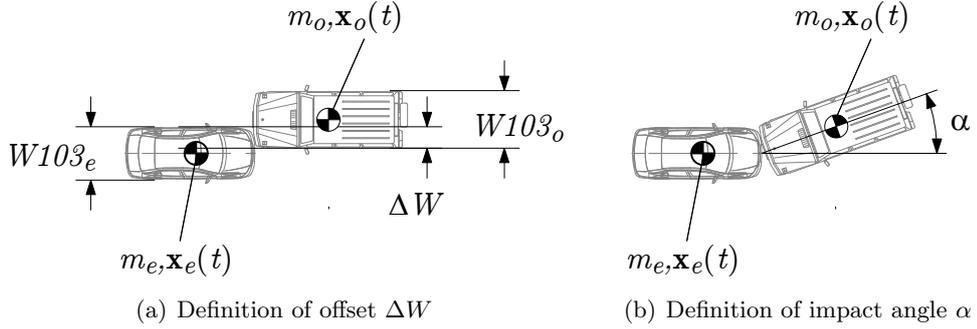
Figure 6.2.: Definition of offset and angle in a frontal impact
