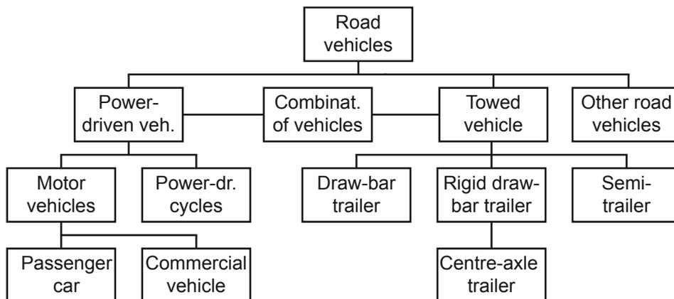
Figure 1.1.: Classification of road vehicles according to DIN 70010, [Nor01]
