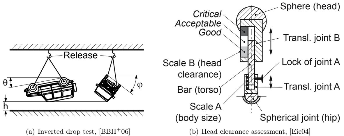
Figure 6.19.: Proposed evaluation of roof strength in rollover
