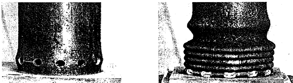
Fig. 2. Yielding steel elements in the laboratory test; left: at the beginning of buckling, right: after approx. 120 mm of axial deformation
