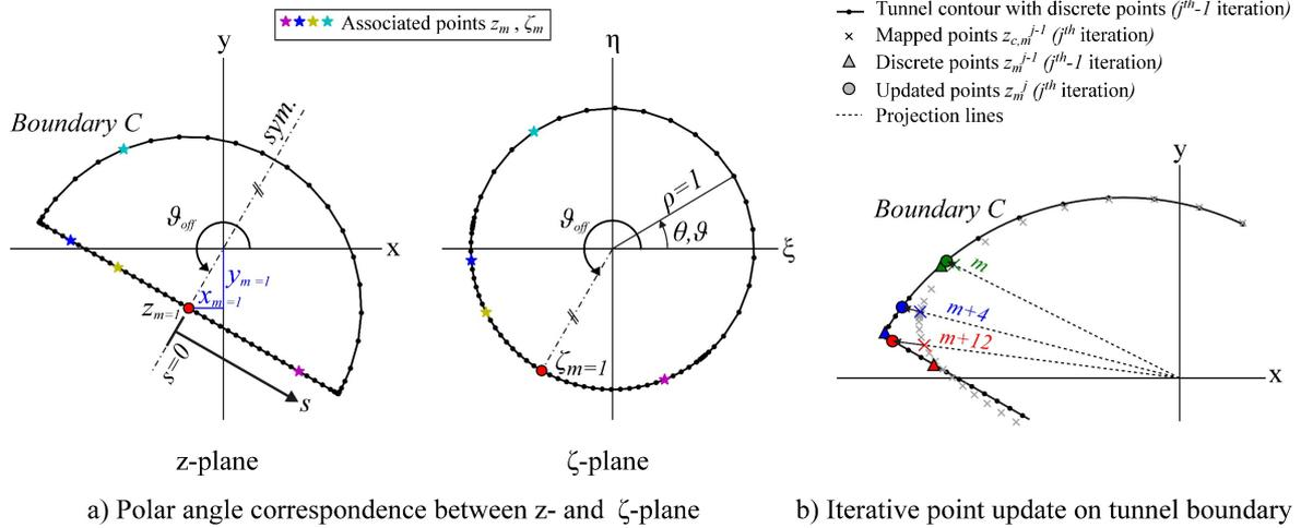
Figure 2. a) Polar angle correspondence for points  $\zeta_m$  in the  $\zeta$ -plane based on the normalized path coordinate  $s$  of points  $z_m$  in the the  $z$ -plane and b) Update of tunnel boundary points  $z_m$  based on the principle of corresponding point polar angle Equality (PCPPAE) after He et al. (2022) by polar projection of points  $z_{c,m}$  onto boundary  $C$  within a single iteration step  $j$  (Exemplarily shown for three points with varying index  $m$ ).
