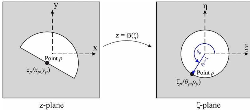
Figure 1. Conformal mapping of points from the physical  $z$ -plane onto the unit circle exterior in the  $\zeta$ -plane.
