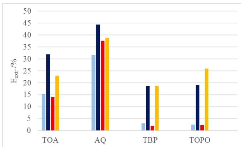
**Fig. 2.** Extraction efficiency for the tested extractants in 1-octanol,  $\text{pH}_{\text{initial}} = 4.88$ ,  $T = 25\text{ }^{\circ}\text{C}$ , red lactic acid in *GF*, yellow acetic acid in *GF*, light blue lactic acid in *XF*, dark blue acetic acid in *XF*.
