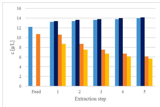
**Fig. 4.** Acid concentrations in the feed and raffinate of the five extraction steps. Light blue = lactic acid in the respective input stream; dark blue = lactic acid in the respective raffinate stream; orange = acetic acid in the respective input stream; yellow = acetic acid in the respective raffinate stream; phase ratio = 1,  $T = 25\text{ }^{\circ}\text{C}$ , solvent phase: TOPO/1-octanol.
