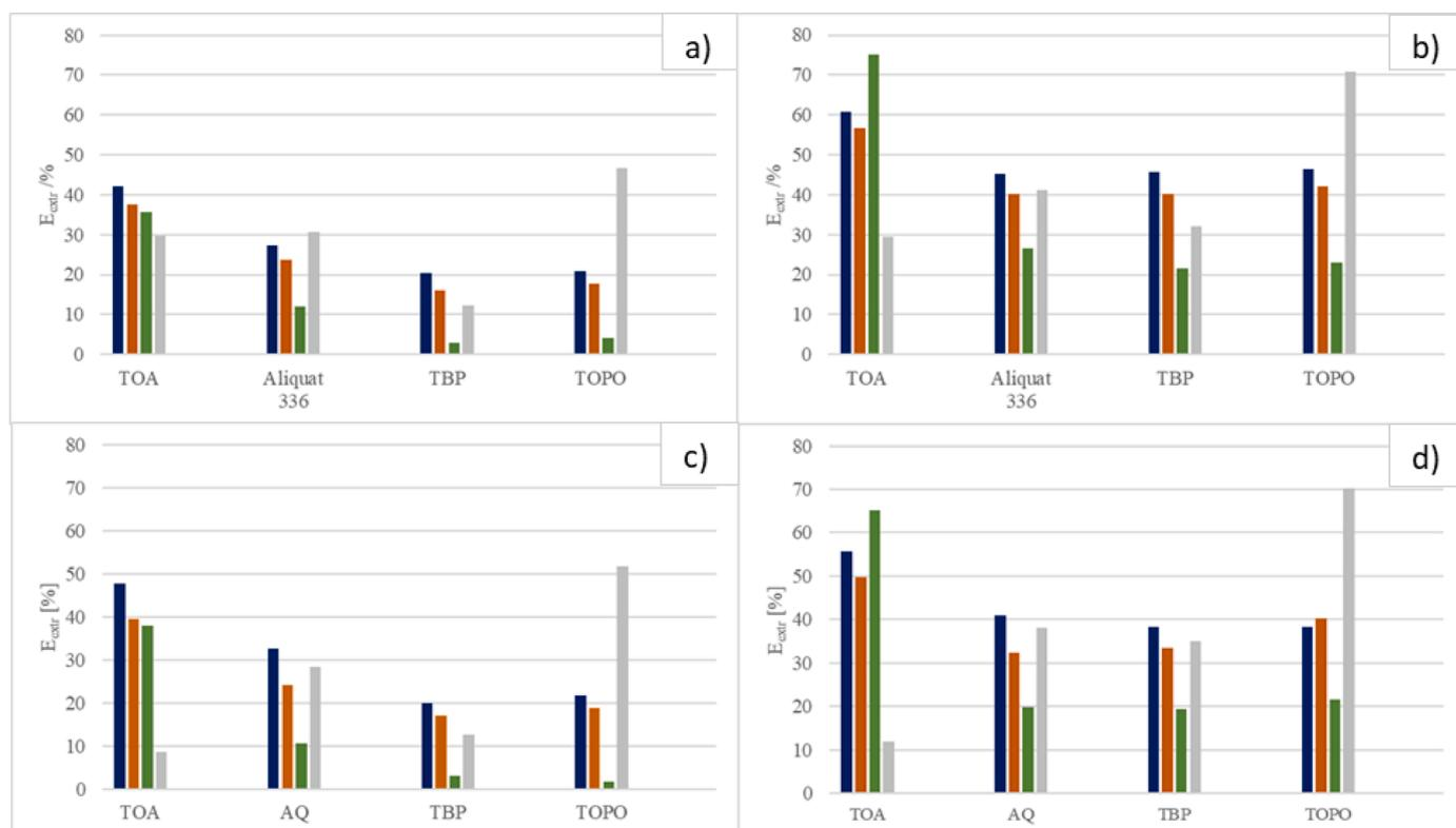
**Fig. 3.** Extraction efficiency for the different modifiers in the *XF*, a) lactic acid and b) acetic acid, and in the *GF* c) lactic acid and d) acetic acid. Dark blue = 1-octanol; orange = 1-decanol; green = DES (33% thymol, 65% menthol); grey = *d*-limonene.  $\text{pH}_{\text{initial, XF}} = 2.57 \pm 0.04$ ,  $\text{pH}_{\text{initial, GF}} = 2.51 \pm 1.18$   $T = 25\text{ }^{\circ}\text{C}$ .
