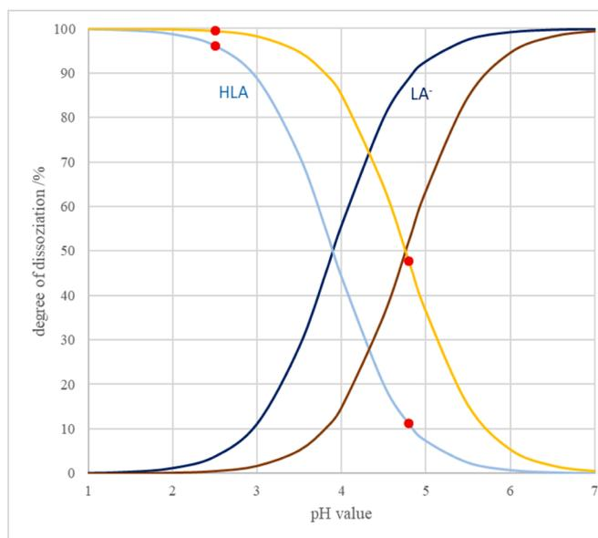
Fig. 1. Haegg diagram for lactic acid, pKa = 3.86 [30], in light blue HLA and in dark blue LA<sup>-</sup>, and acetic acid pKa = 4.75, orange HAA, brown AA<sup>-</sup>; red dots for the two pH values investigated; 4.8 = fermentation broth; 2.57 ± 0.04 adjusted pH value.
