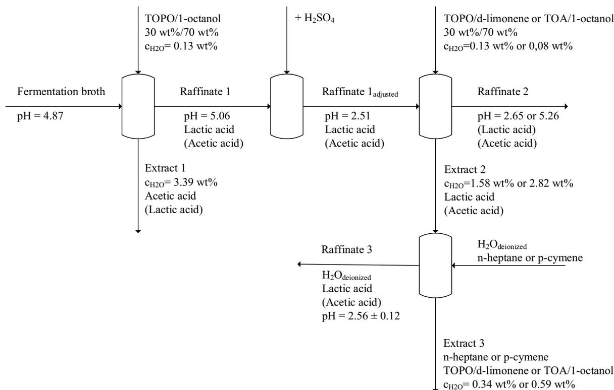
**Scheme 1.** Schematic of the two-step extraction and back extraction. Compounds given in brackets mean that small quantities thereof are expected, e.g. extract 1 consists mainly of acetic acid, but small amounts of lactic acid are expected, the same applies to the other streams.
