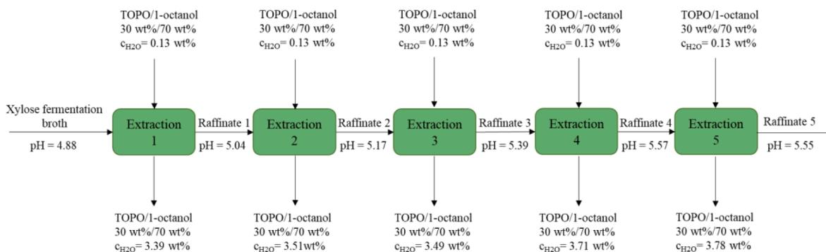
**Scheme 2.** Schematic of the five-step extraction.
