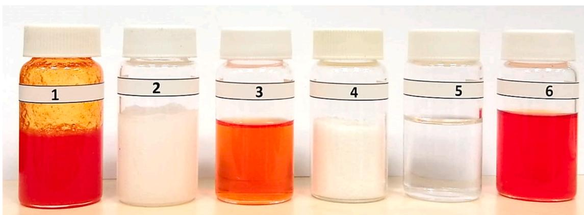
Fig. 7. Intermediate and final products of the experimentally evaluated process in continuous mode, 1) feed, 2) wet, refined salt, 3) extract, 4) dried refined salt, 5) recycled solvent, 6) organic residue (glycerol), colouring agent: methyl red.
