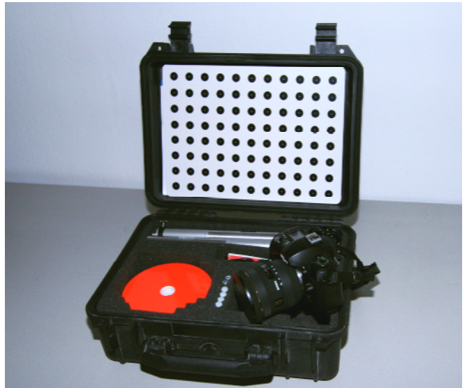
Fig. 9: Picture of the ShapeMetriX3D calibrated camera together with reference elements and calibration target.
