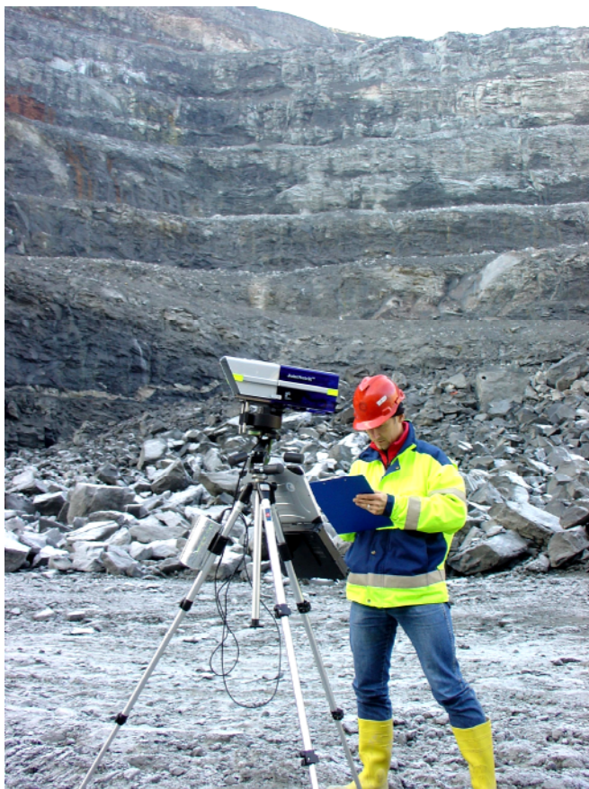
Fig. 11: Application of the JointMetriX3D system in a large open pit mine in Sweden.
