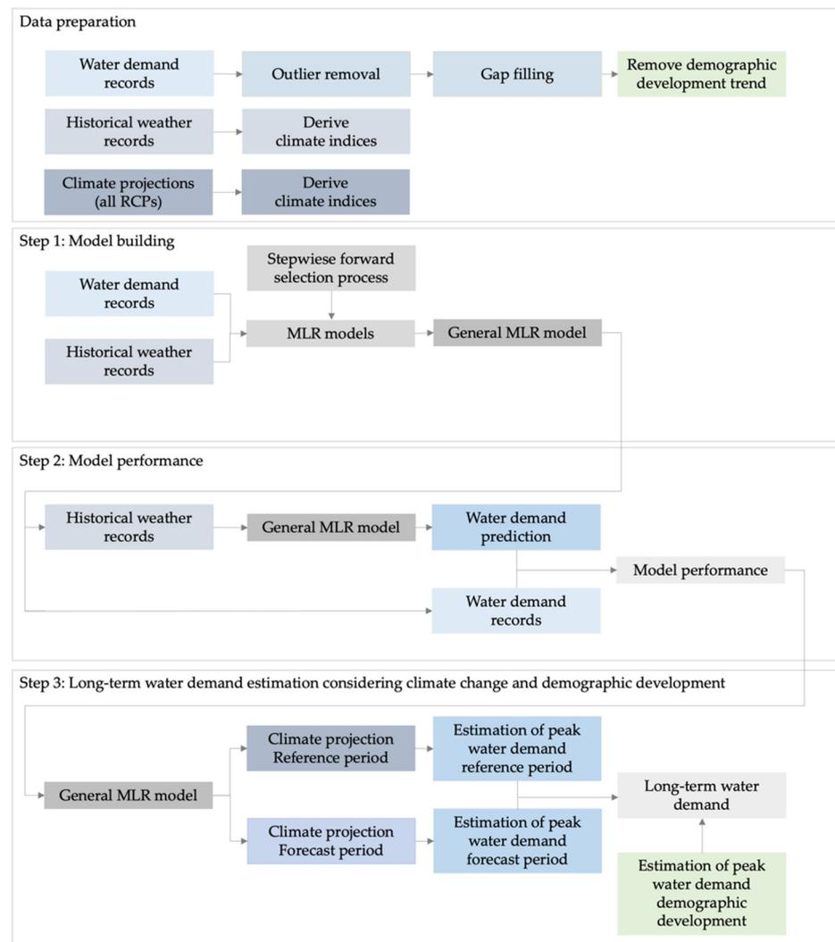
**Figure 2.** Model building workflow. The first step is data preparation. The modeling process is divided into three steps. The first is model building, the second is model performance assessment, and the final step is long-term peak water demand estimation.
