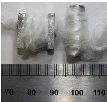
**Fig. 4** Filament on carrier bodies, after a dry experiment
