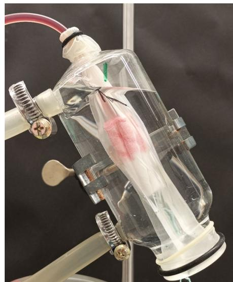
**Fig. 1** Syngina setup with tested sample in the middle, liquid supply from the top and 27 °C deionized water surrounding the sample
