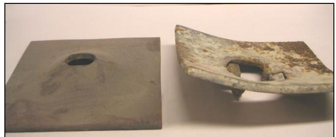
Fig. 7. Bolt plate before installation (left) and failed punched through bolt plate.
