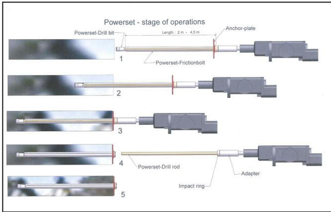
Fig. 9. Self-drilling installation procedure (five stages).
