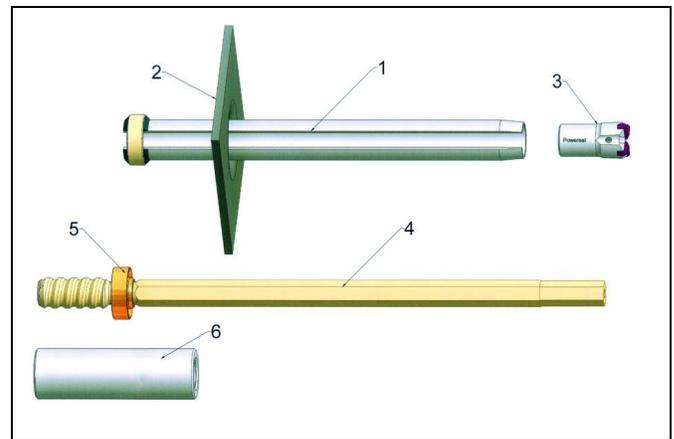
Fig. 8. Components of the Power Set rock bolt system (caption: 1 -Power Set bolt; 2 - anchor plate; 3 - drill bit; 4 - drill rod; 5 - impact ring; 6 - adapter coupling).
