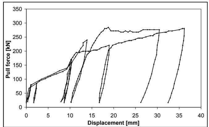
Fig. 17. In-situ pull tests – Edgar Experimental Mine 2.
