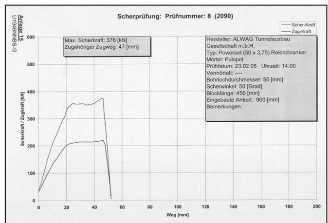
Fig. 13. Laboratory test – combined tensile-shear test  $50^\circ$ .
