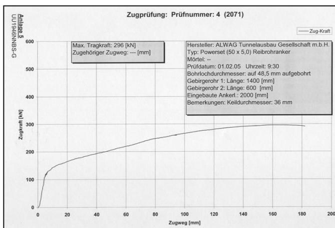
Fig. 11. Laboratory test – tensile pull test.
