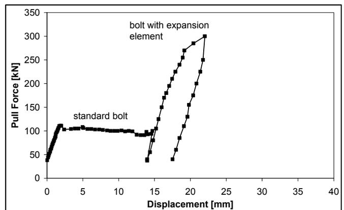
Fig. 18. In-situ pull tests – Esmeralda Mine.
