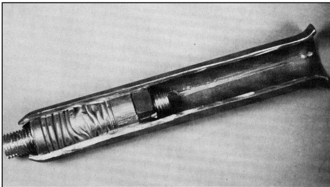
Fig. 4. Cross-sectional profile of a bolt head with buckling tube from Ingenieure Mayreder, Kraus Co. [5].
