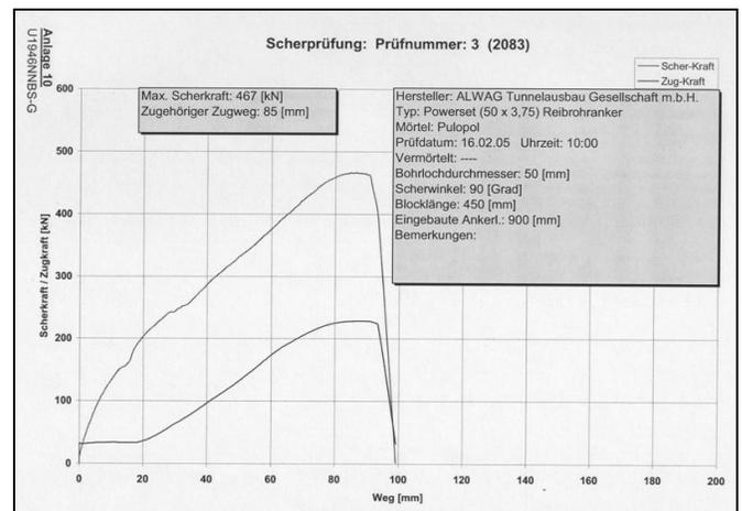
Fig. 12. Laboratory test – combined tensile-shear test  $90^\circ$ .
